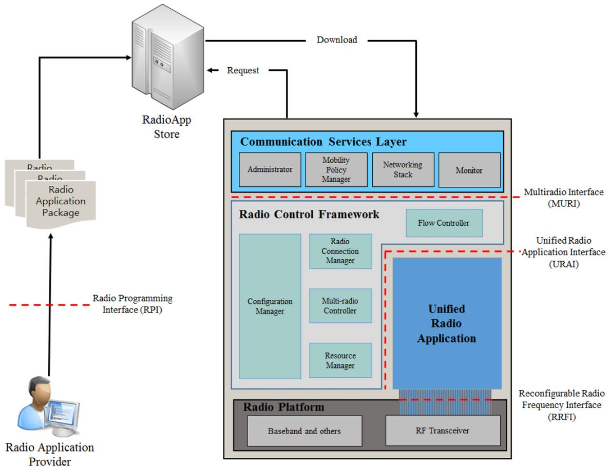
**Figure 4: Standard reconfigurable mobile device architecture and related interfaces**
