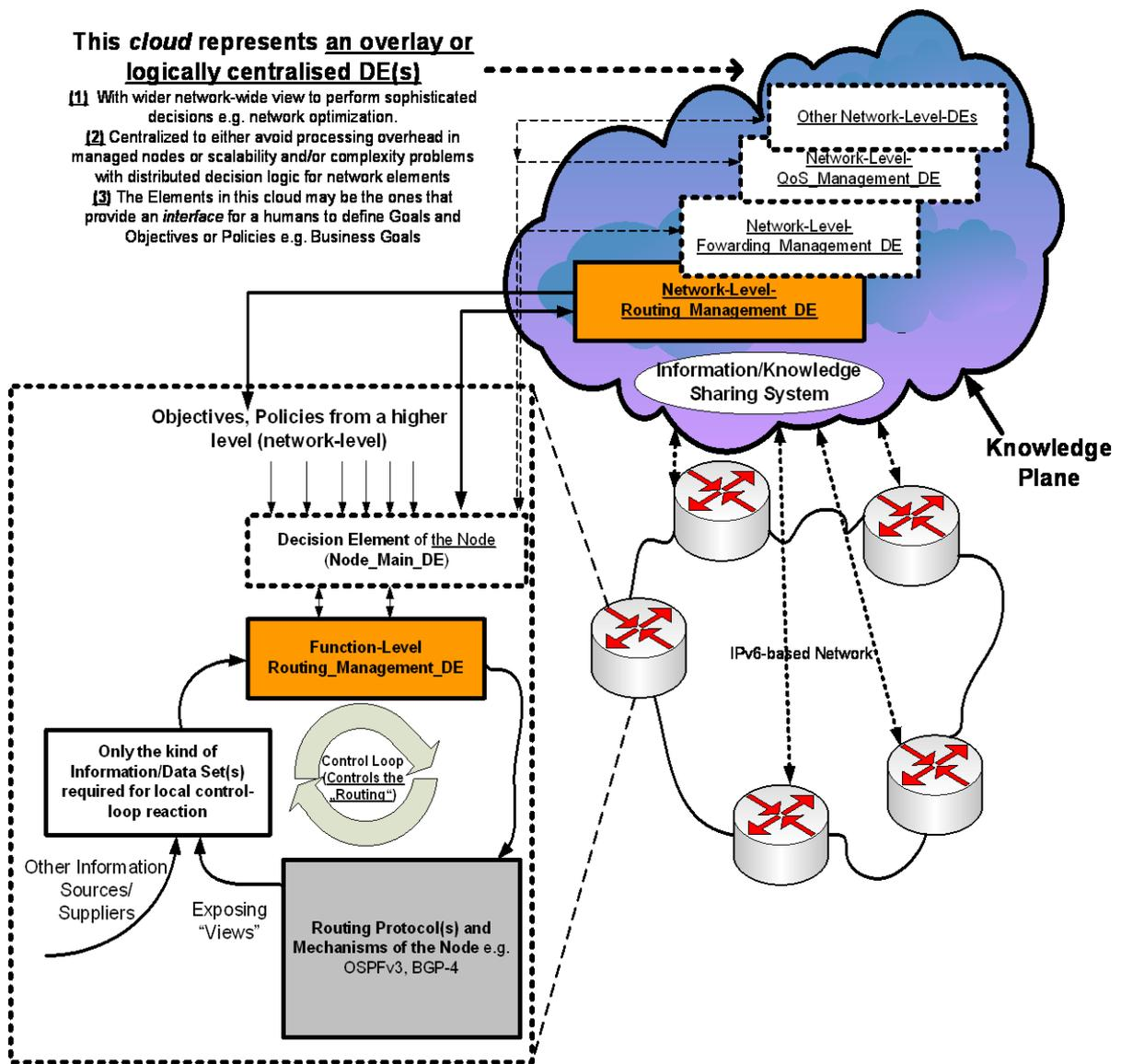
**Figure 3: Illustrating the interworking of fast control-loop and slower control-loop for routing management (can be applied both to IPv6 and IPv4 environments)**
