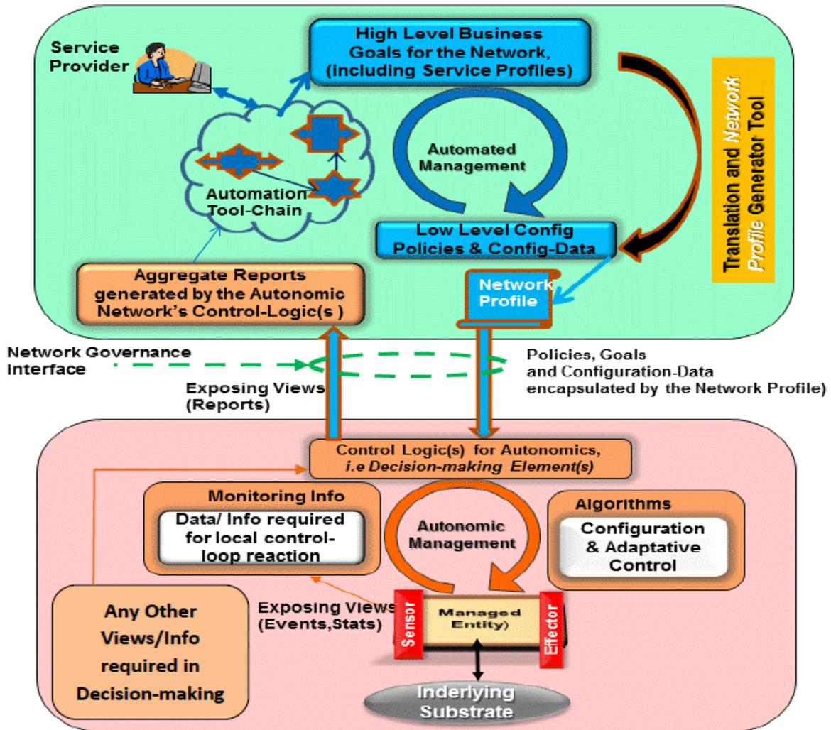
Figure 1: Automated Management vs Autonomic Management illustration (their interaction and complementarity)
