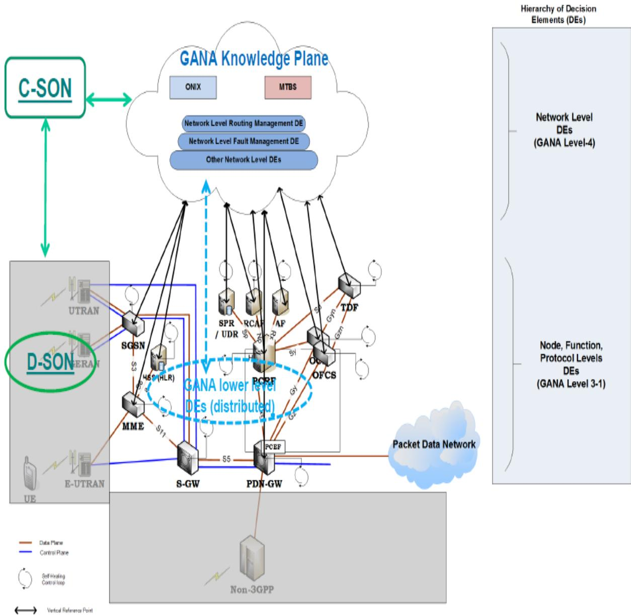
**Figure 4: Instantiation of the GANA Knowledge Plane for the 3GPP EPC Core Network, and the need for EPC KP to interwork with 3GPP C-SON (figure extracted from [28])**
