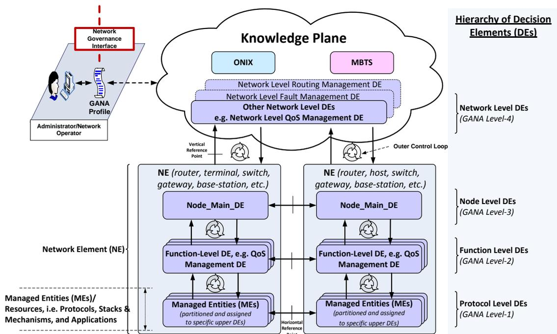
Figure 2: Snapshot of the AFI GANA Reference Model
