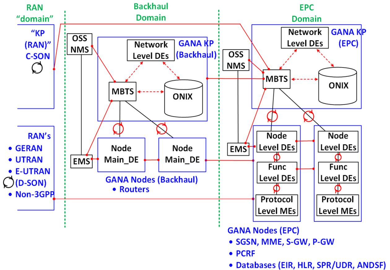
Figure 5: Interactions involving C-SON, and GANA entities for 3GPP Core Network and backhaul, to enable E2E Self-Optimization across network segments (figure extracted from [28])
