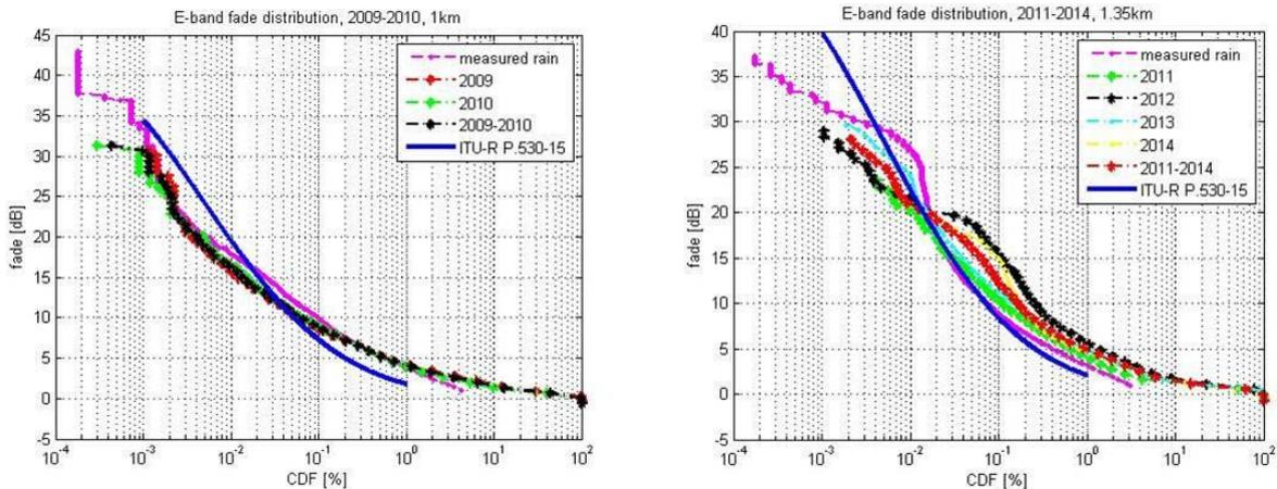
Figure 6: Fade statistics: a) 2009-2010 for Link 1, b) 2011-2014 for Link 2.
