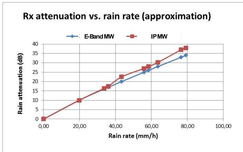
**Figure 10: Rain rate vs. rain attenuation (approximation)**
