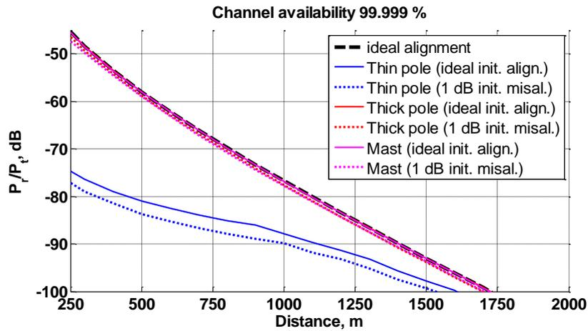
Figure 55: Link budget vs. Distance for availability level 99.999% (frequency 75 GHz, HPBW = 2 deg.).
