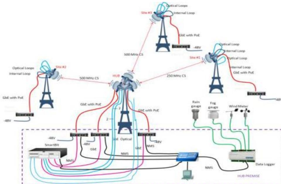
**Figure 11: E-band Trial configuration**
