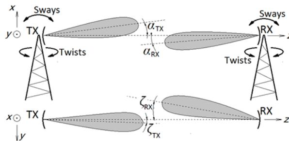
Figure 50: Illustration of twist and sway movements in vertical structure seen from side (upper picture) and from top (lower picture).
