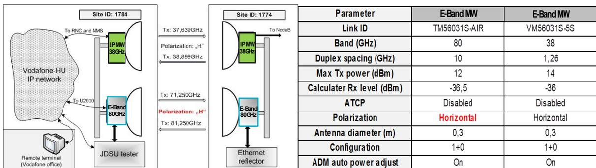
Figure 8: Trial configuration and RF parameter setting
