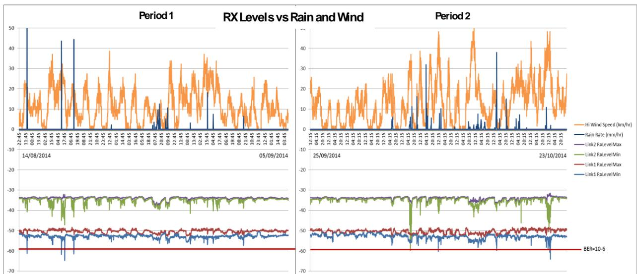
Figure 28: Correlation between rain rate and wind levels with the Rx levels
