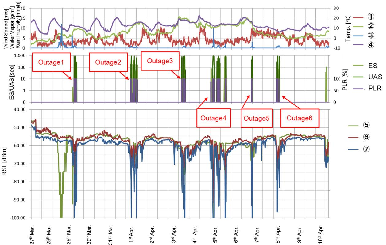
Figure 24: Sample of measured data at Site A for setup ② (+12dBm Tx power).
