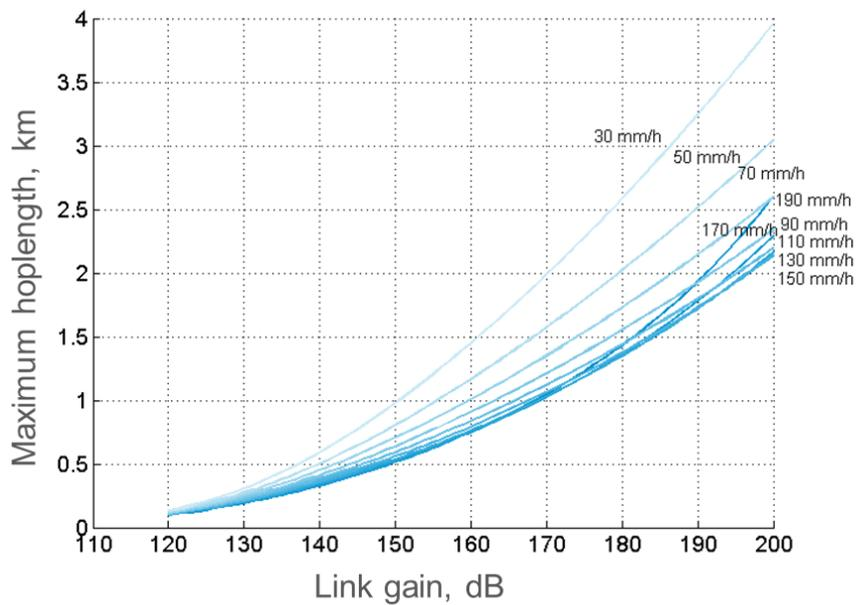
Figure 2: Maximum hop length with 143 GHz carrier for different rain intensities.
