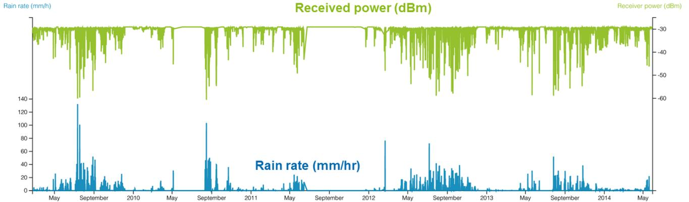
Figure 5: Received power versus rain intensity.
