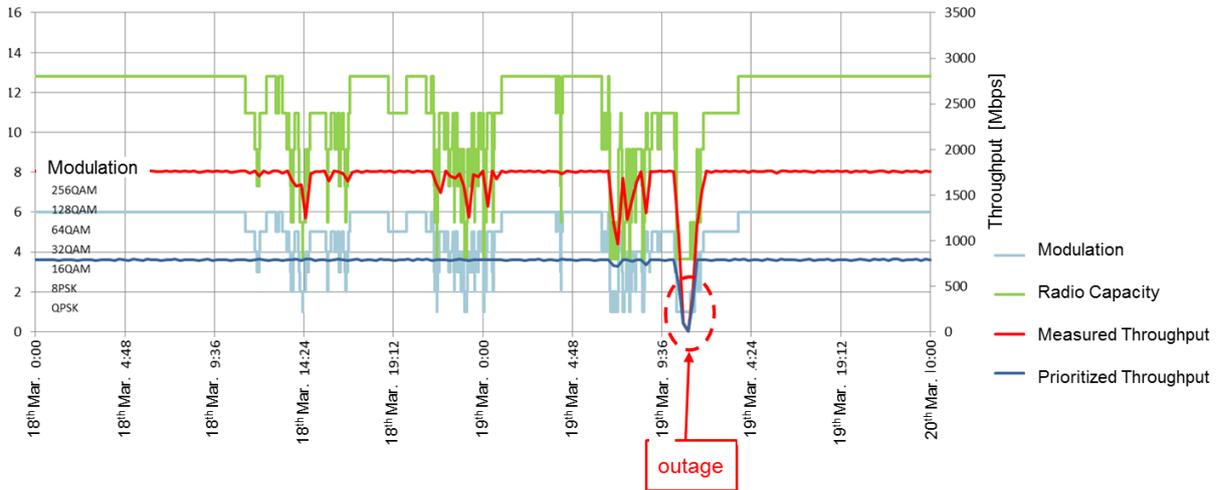
Figure 20: Detail view of fading event
