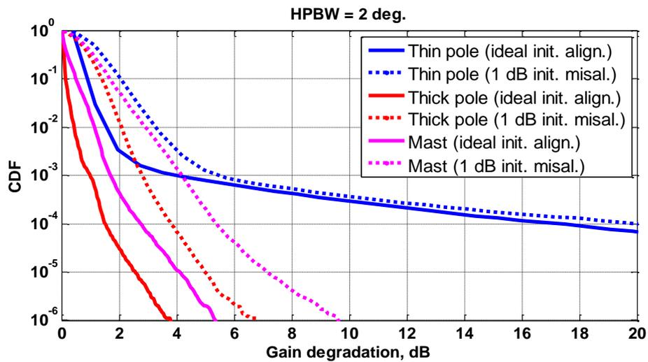
**Figure 54: CDF attenuation due to deflections (three types of sites, HPBW = 2 deg.).**
