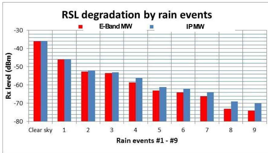
Figure 9: Comparison of rain attenuation (38GHz “H”, 80GHz “V”)
