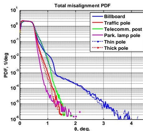
Figure 51: PDFs of total antenna misalignment for HPBW 1°.
