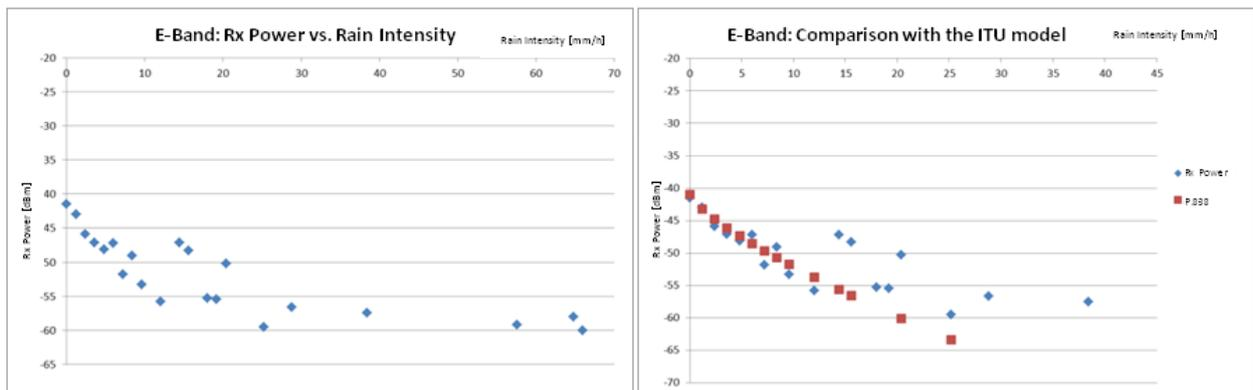
Figure 14: E-band system rainfall class vs. Rx power
