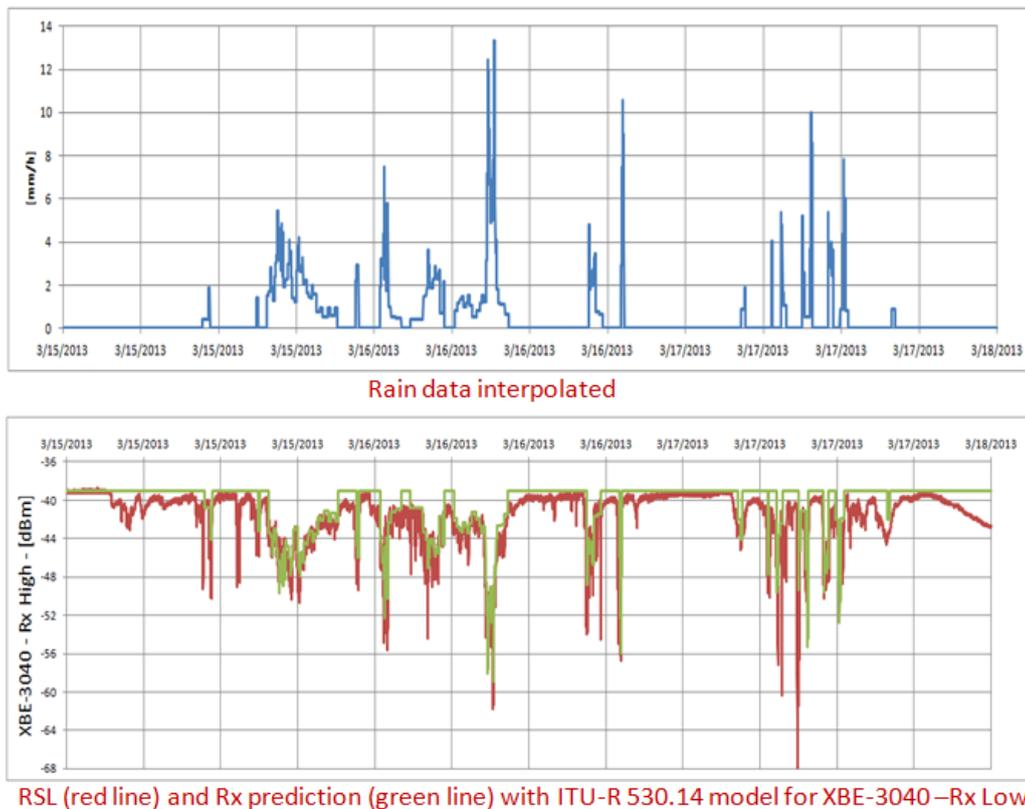
Figure 12: Instantaneous rain rate and corresponding attenuation along one of the hops in the trial
