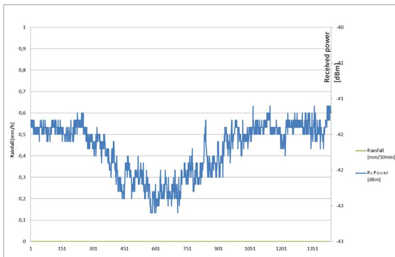
Figure 16: No rain events, E band system in normal operation
