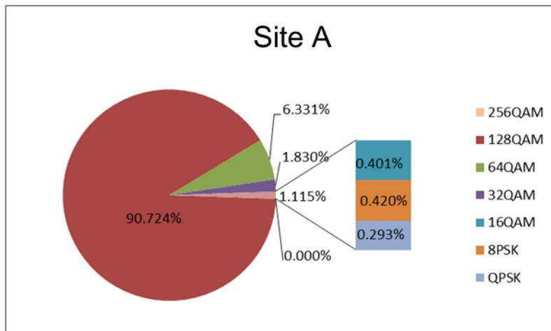
Figure 21: ACM modes usage profile from the trial
