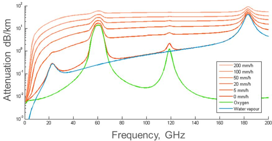
Figure 1: Path attenuation in LOS at different rain intensities.
