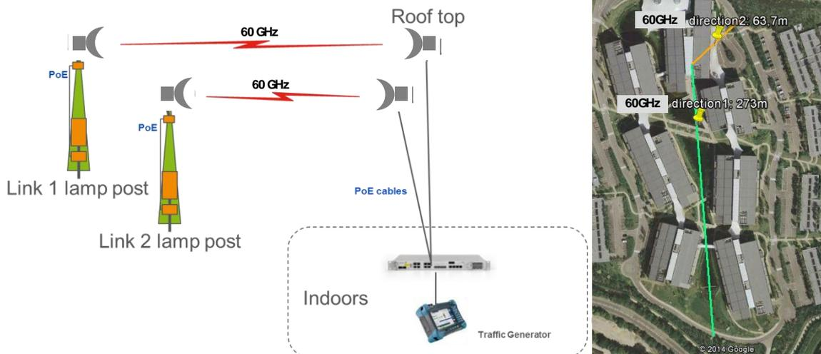
Figure 27: Trial setup
