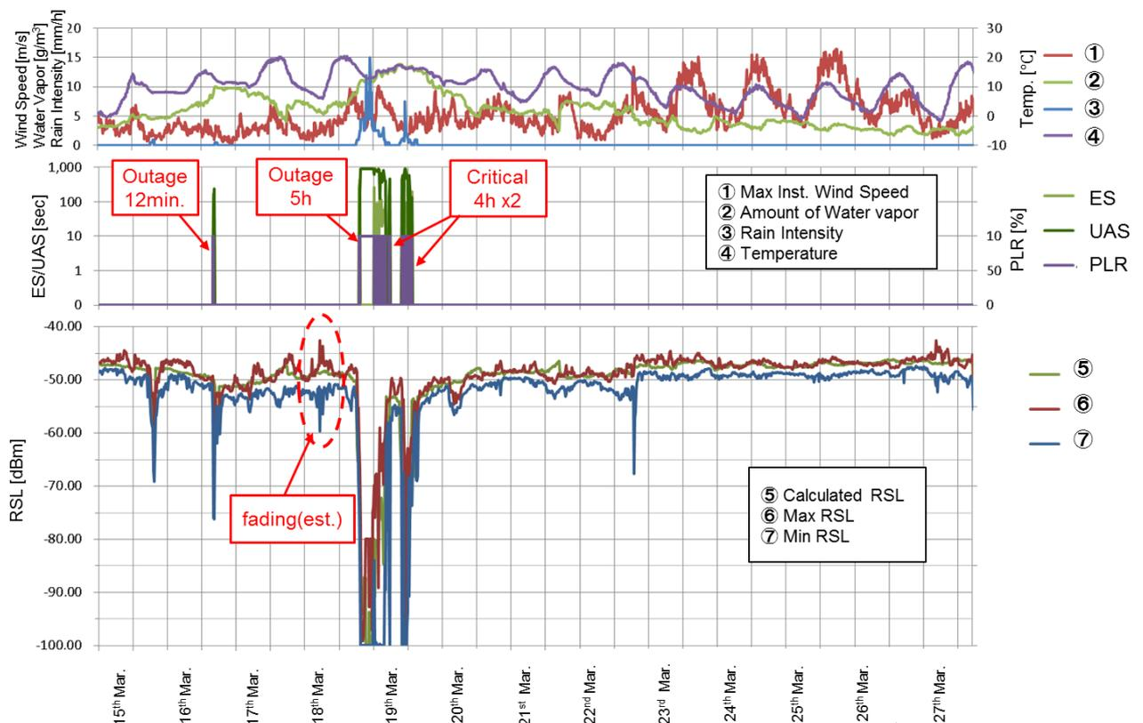
Figure 23: samples of measured data at Site A with setup ① (+18dBm Tx power).
