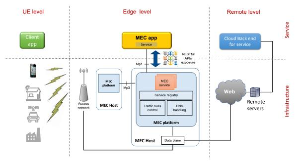
Figure 2: MEC applications, interaction and service exposure
