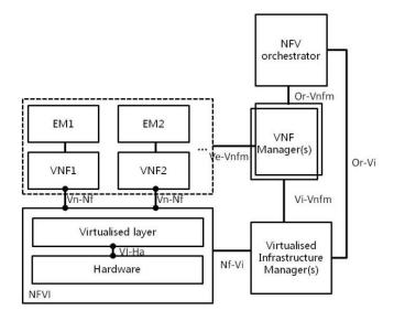
Figure 5: ETSI NFV reference architecture (ref. ETSI GS NFV 002 [49])
