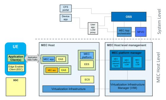
Figure 3: High-level overview of synergized MEC architecture in virtualized environments
