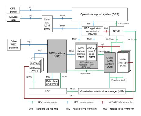
Figure 4: Reference architecture variant for MEC in NFV (ref. GS MEC-003 [1])
