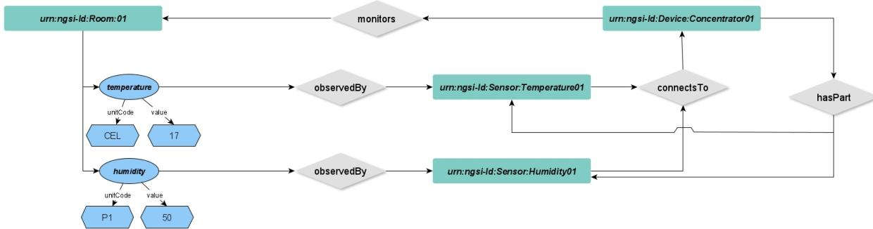
**Figure 7: Modelling a Concentrator Device in NGSI-LD**
