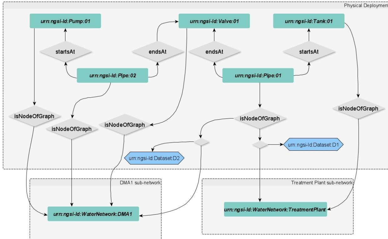
**Figure B.7: Modelling Water Network Topology using endograph Relationship**
