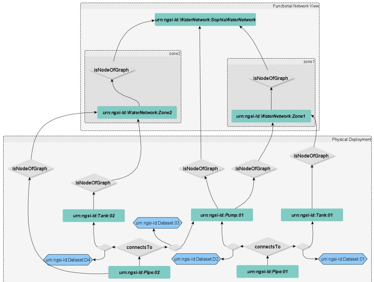
Figure B.13: Modelling the use case example using the recommended NGSI-LD ontology
