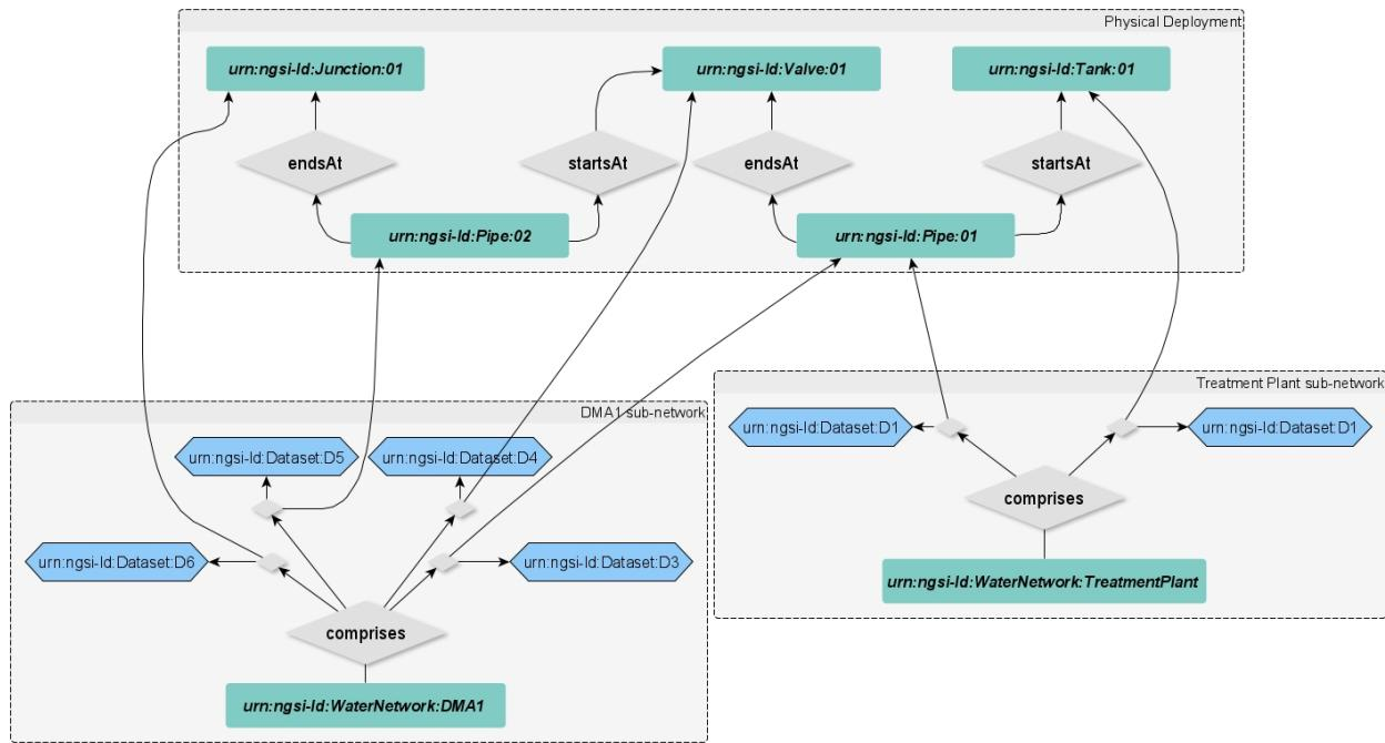
Figure B.8 Modelling Water Network Topology using `comprises` Relationship
