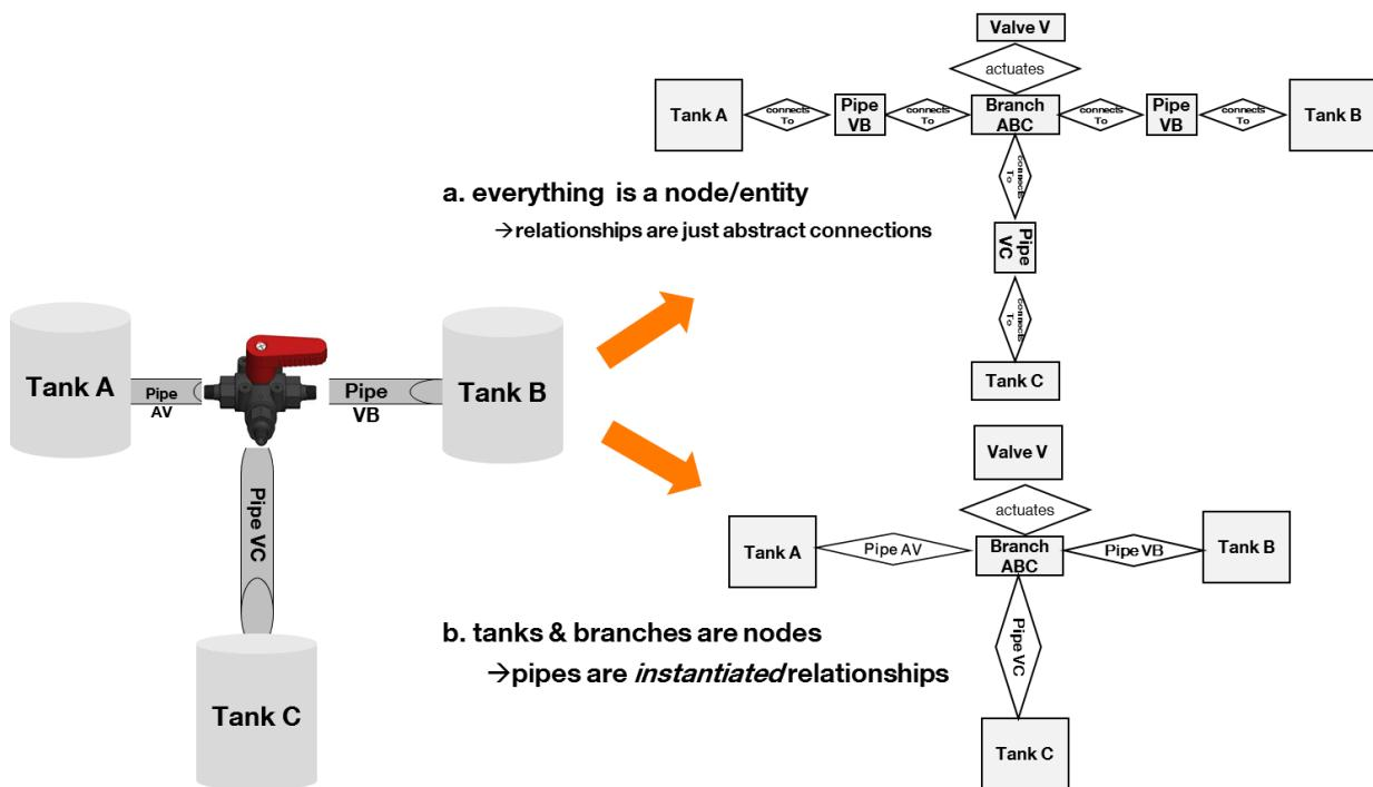
Figure 5: Example of relationship used to model a physical connection in a water network
