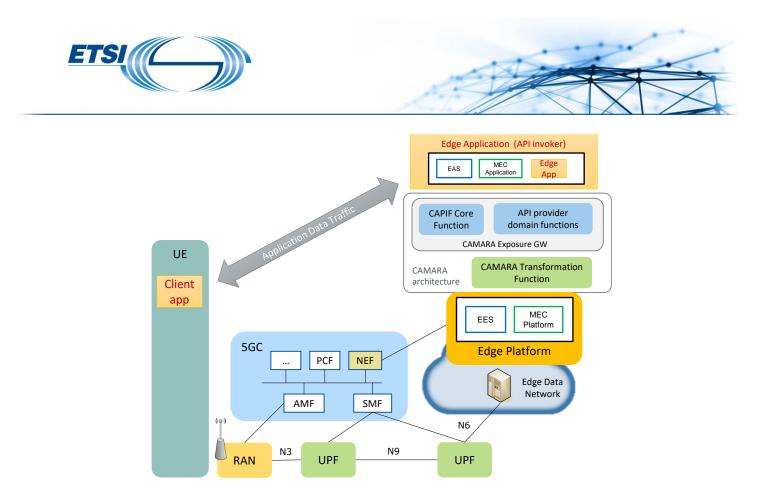
Figure B.3: Option for Edge Native applications to consume MEC services in a MEC federation (via CAPIF framework and the CAMARA architecture).
