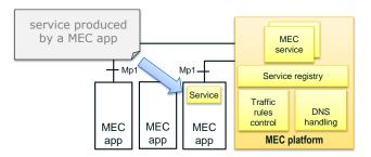
Figure 7: A MEC application instance may consume and/ or produce MEC services
