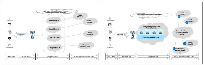
Figure 1: Edge Enterprise scenarios: (left) traditional multi-Cloud implementation; (right) leveraging Common Edge Native Platform and virtual common Cloud.
