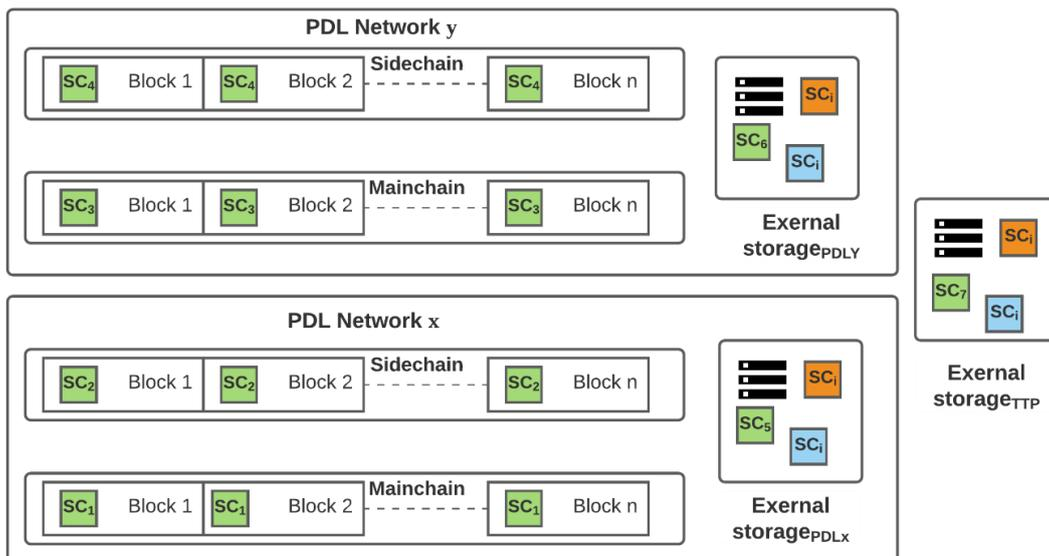
Figure 4: Modularized Smart Contract (Source: ETSI GS PDL-011 [10])
