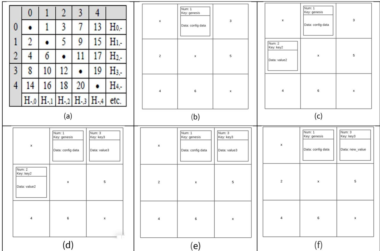
Figure 10: Blockmatrix Structure and Hyperledger Fabric Implementation
