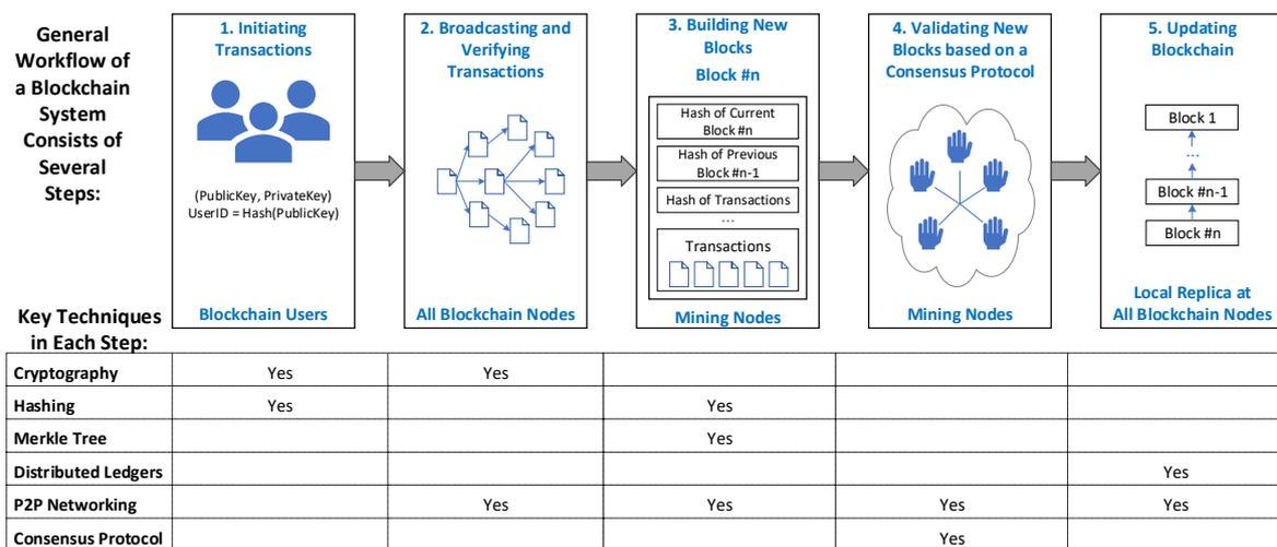
**Figure 1: General Workflow of a Blockchain System**
