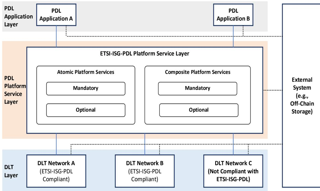
Figure 2: ETSI-ISG-PDL Reference Architecture (Source: Adapted from draft ETSI GS PDL-012 )
