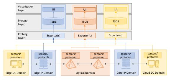
Figure 24: The energy monitoring system
