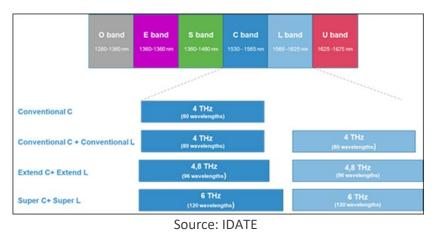
Figure 11: Different wavelengths of fibre optical communication band
