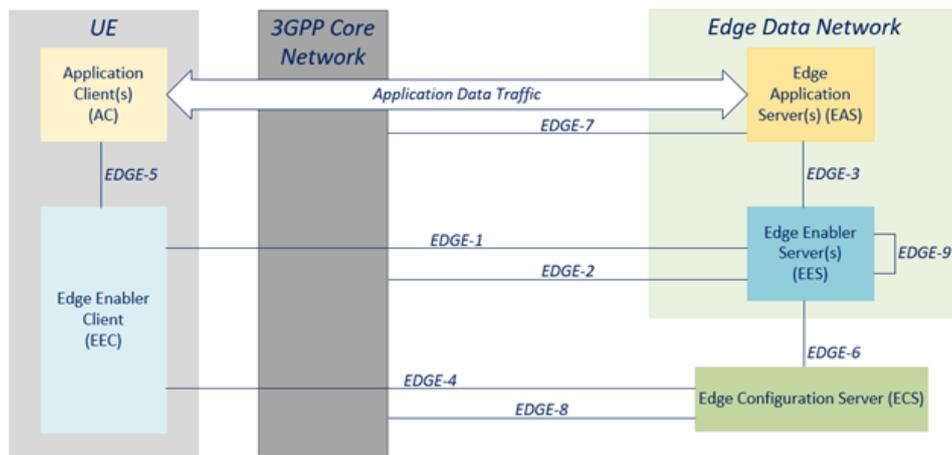
**Figure 6: Architecture for enabling edge applications [TS23.558]**
