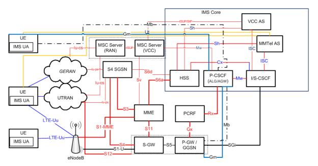
Figure 1: IMS/LTE Basic Configuration
