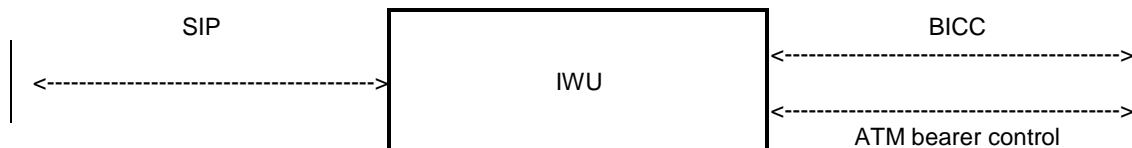
Figure 2: Interworking between SIP and BICC
