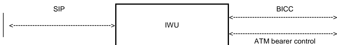
Figure 2: Interworking between SIP and BICC
