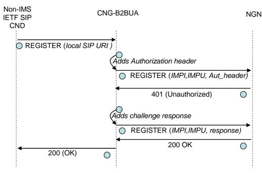
Figure 8.5: Non IMS capable device Authentication trough CNG SIP Proxy
