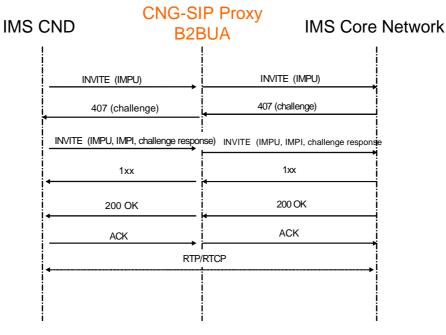
Figure 8.8: Outgoing call IMS capable device
