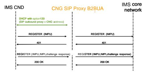
NOTE: This scenario is not possible in case of IMS device implementing the AKA authentication mechanisms (IPsec tunnel through the CNG).
