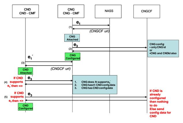
Figure 8.2: Management flow with CNG routed mode
