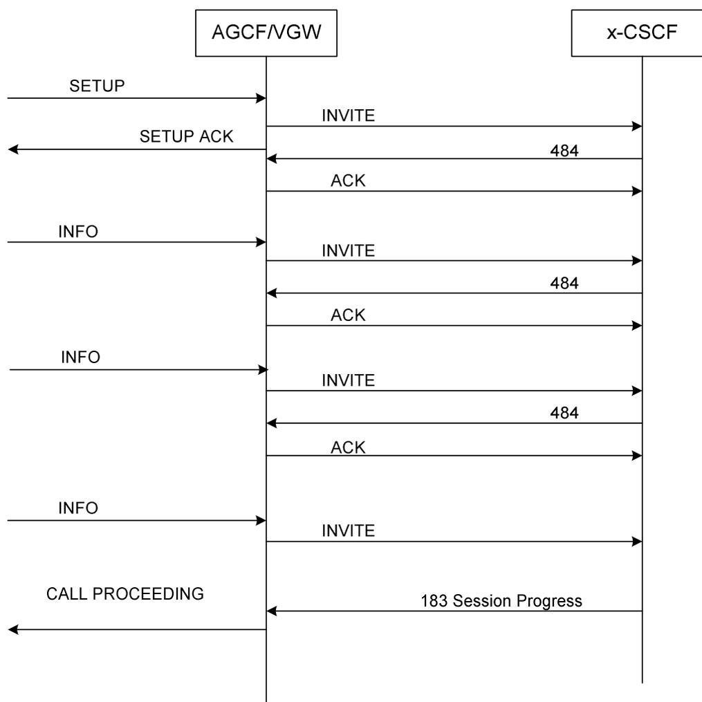
Figure D.1.1.3-7: 484 message without Min-length X parameter
