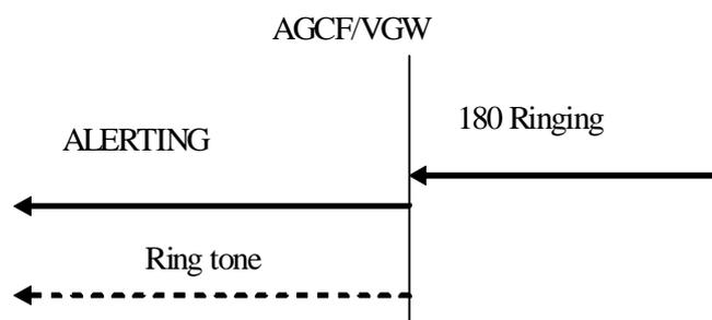
**Figure 5.1.1.2.1.0-1: Sending of ALERTING (Receipt of first 180 Ringing without authorization of early media)**
