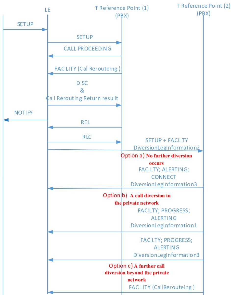
**Figure 5.2.5.2.3-1: Simplified message flow for response to a call setup in case of call forwarding**
