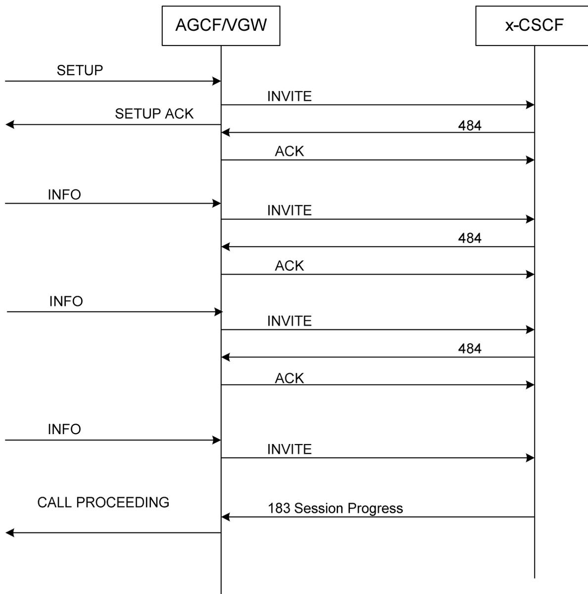
Figure D.2.1.2-7: 484 message without Min-length X parameter
