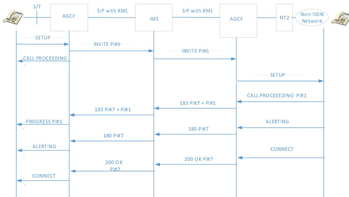
Figure H-2: Interworking situation IMS, an ISDN (PES) user is calling an ISDN (PES) user
