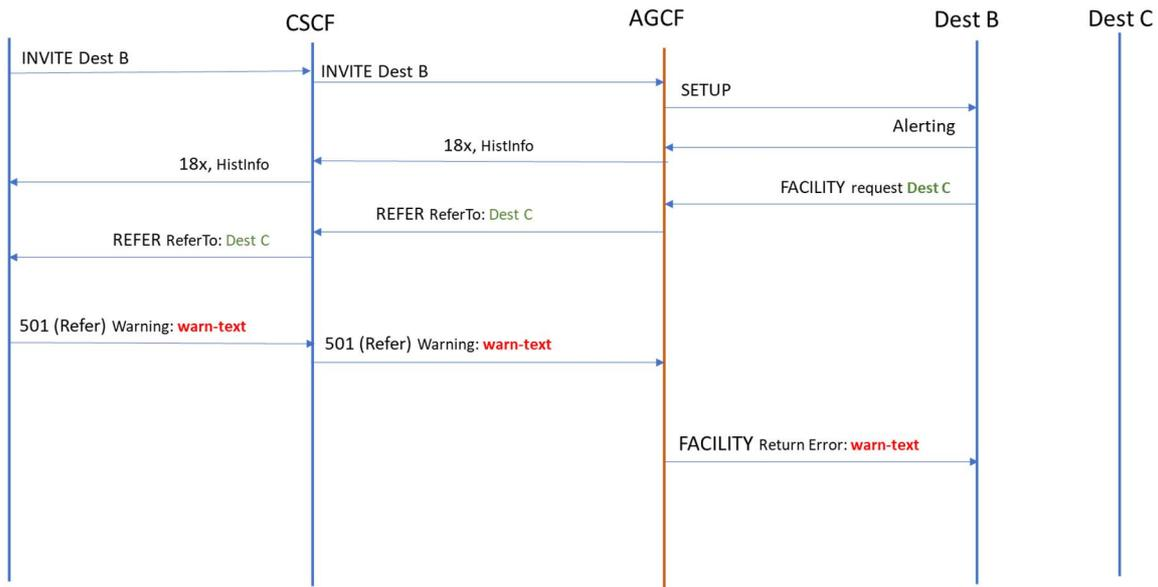
Figure 5.2.5.2.4-2: Partial Rerouting Option B unsuccessful
