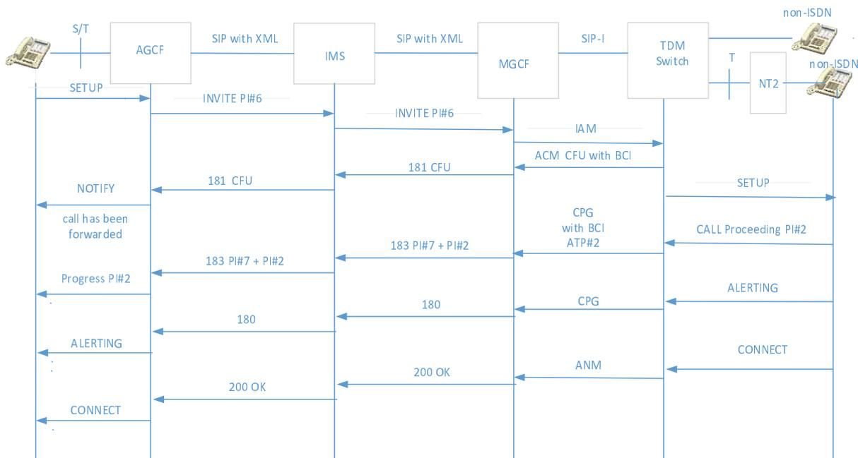
**Figure H-5: Interworking situation IMS to TDM, an ISDN (PES) user is calling a non-ISDN user which forwarded the call to an ISDN user with a PBX which has a non-ISDN access. The ISDN user is in the same switch**
