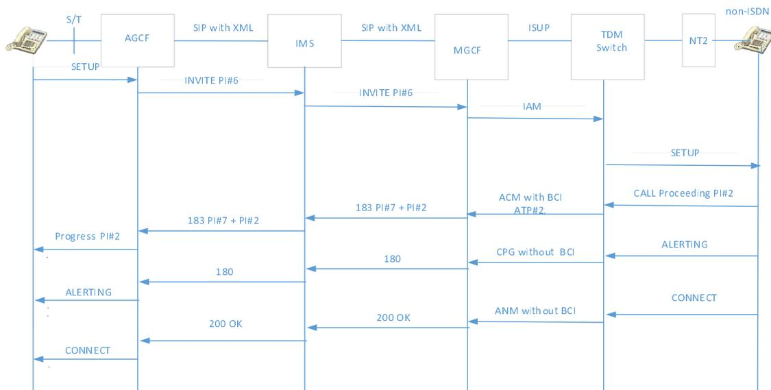
**Figure H-4: Interworking situation IMS to TDM, an ISDN (PES) user is calling an ISDN user with a PBX which has a non-ISDN access**
