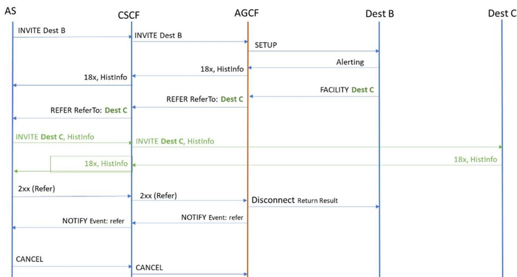
**Figure 5.2.5.2.4-1: Partial Rerouting Option B successful**
