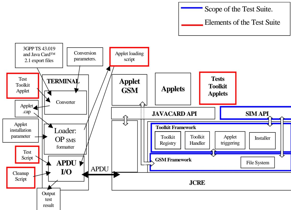
NOTE: Figure 4.2 shows the test architecture required to test interoperability at both API and bytecode level. The latter is currently not included in the current specification. The diagram is for information.
