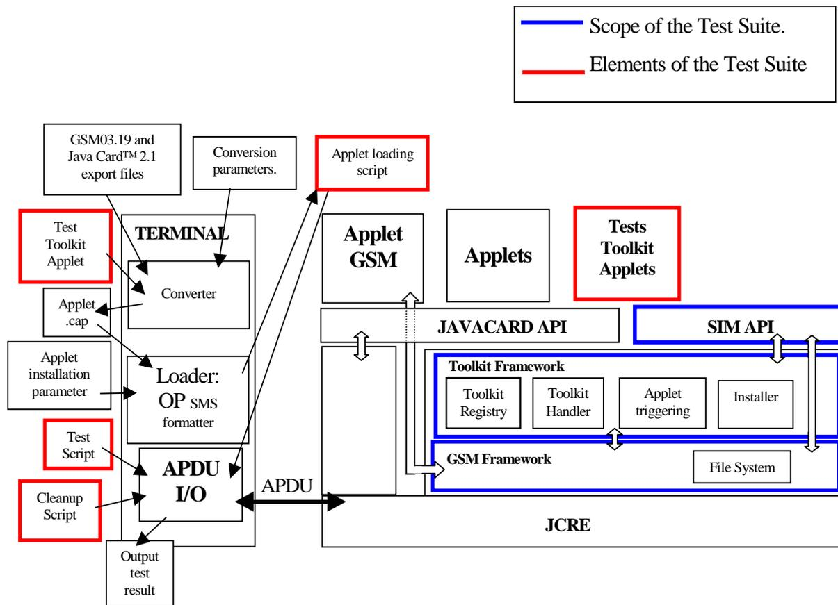
NOTE: Figure 4.2 shows the test architecture required to test interoperability at both API and bytecode level. The latter is currently not included in the current specification. The diagram is for information.
