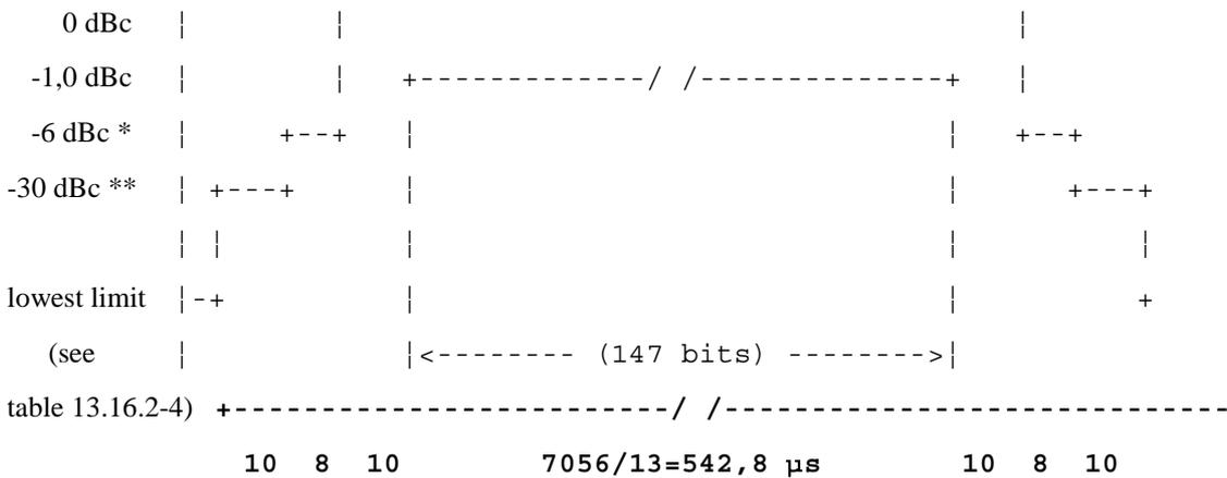
**Figure 13.16.2-1: Power / time template for normal bursts**
