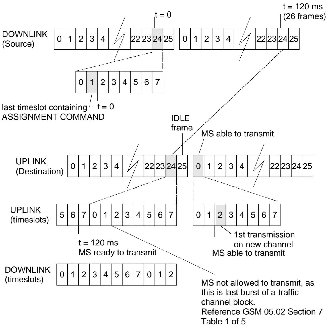
Timing difference between Downlink and Uplink is 3 timeslots.
