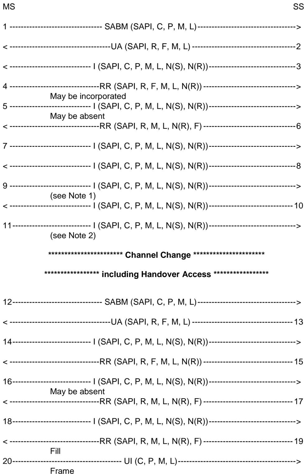
NOTE 1: The MS may send RR frames on the FACCH in addition to the I frames in 9 and 11.
