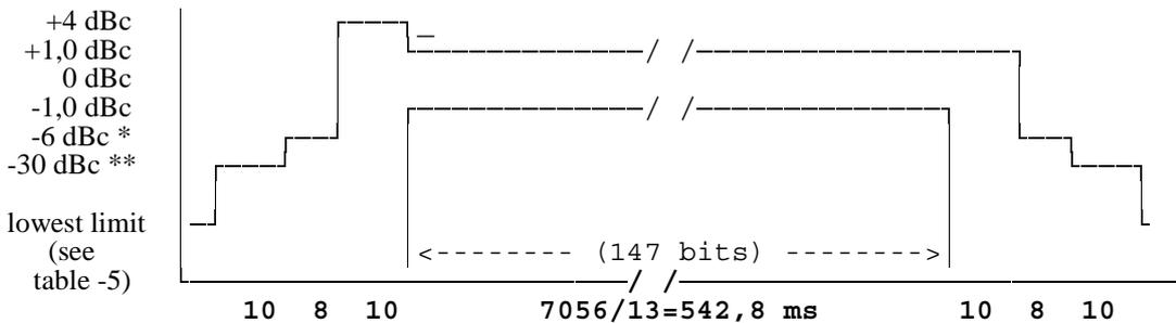
**Figure 13-1: Power / time template for normal bursts**
