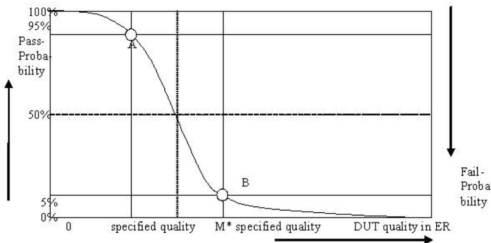
Figure A7.2.3.6: Pass probability versus DUT quality
