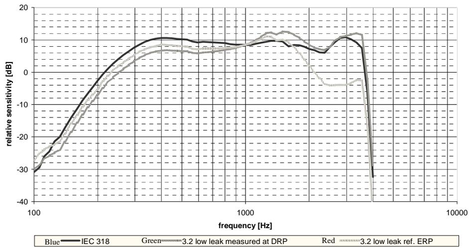
This slide as well as the following two shows results of three measurement and evaluation methods per each mobile sample. The blue curve is as measured sealed to IEC 318 closed coupler. The green curve is as measured with type 3.2 low leak coupler at DRP. The red curve shows the same measurement data corrected to ERP using the correction function provided by the manufacturer.
