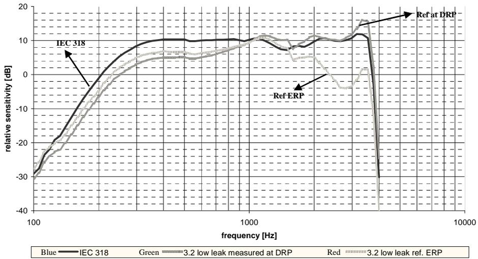
Below 1 KHz both type 3.2 curves are similar. The level decreases from IEC 318 to the type 3.2 results is due to the leak. At high frequencies the measured type 3.2 curve without DRP to ERP correction (green) clearly illustrates better compatibility towards IEC 318 results than the curve referred to ERP (red).
