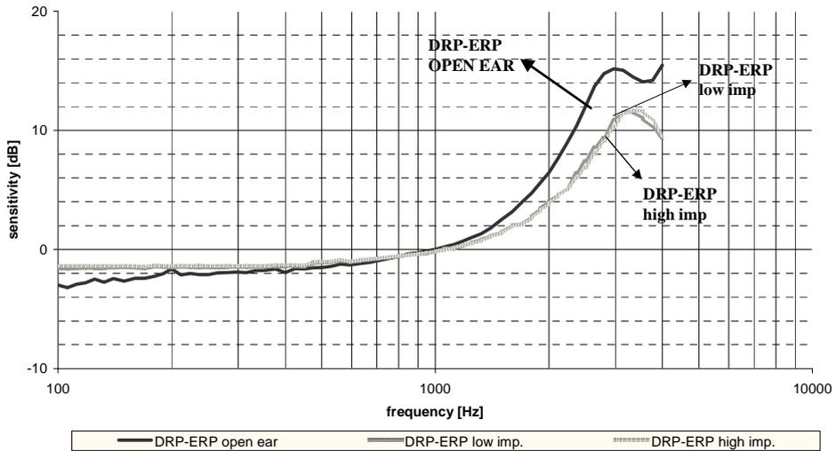
The three curves show the DRP to ERP transfer function for different source conditions. The blue line is obtained mounted in a baffle. The other two functions are measured with a probe microphone at ERP on two mobiles with different acoustic source impedance.
