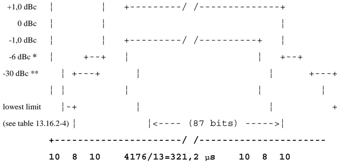
**Figure 13.16.2-2: Power / time template for access burst**
