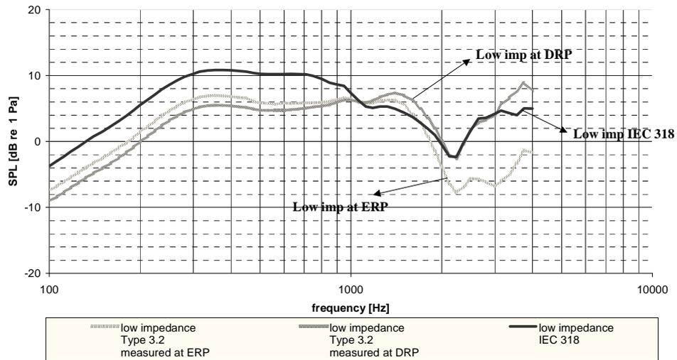
Contrary to the first three slides, the type 3.2 low leak response at ERP here is not calculated, but measured with a probe microphone. The relationship between the three curves is the same as in each of the first three slides.
