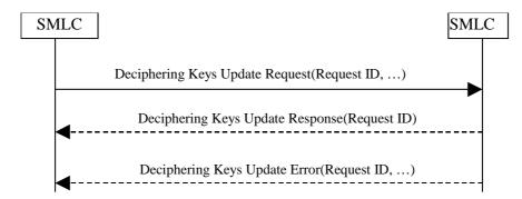
This operation allows a SMLC controlling deciphering keys to send the keys to another SMLC Client.
