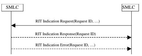
This operation allows a SMLC to send RIT information to another SMLC. It can be used both in the cased of autonomous provision, and the provision of RIT information on request.
