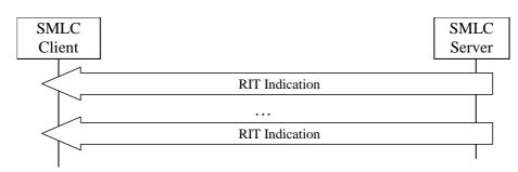
In the autonomous mode the procedure consists of one or more RIT Indication operations.
