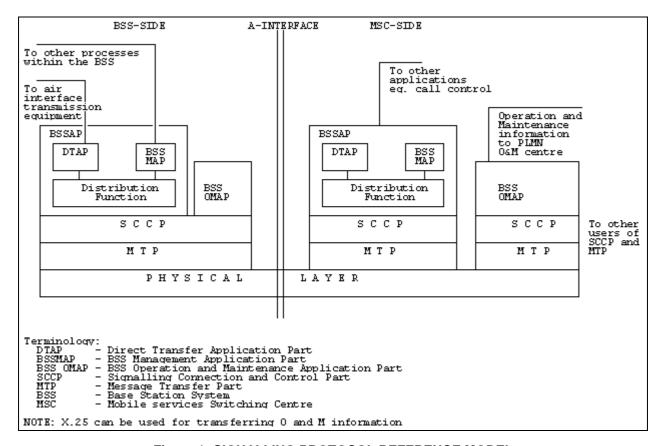
Figure 1: SIGNALLING PROTOCOL REFERENCE MODEL
