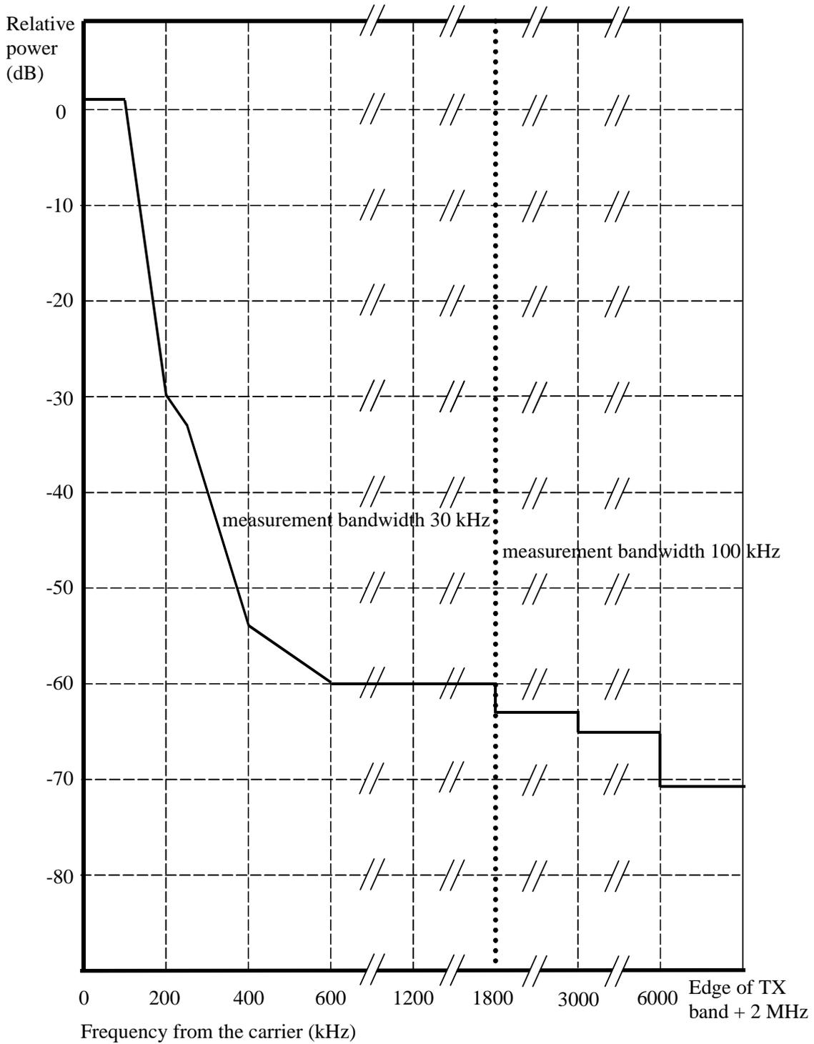
**Figure A.1b: GSM 400, GSM 900, GSM 850 and GSM 700 MS spectrum due to 8-PSK and 16-QAM modulation with normal symbol rate and QPSK, 16-QAM and 32-QAM modulation with higher symbol rate using narrow BW pulse shaping filter**
