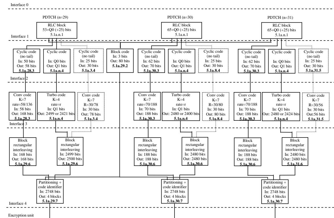
**Figure 1l: Channel Coding and Interleaving Organization for EGPRS2-B Downlink Packet Data Channels, DBS-10 to DBS-12**
