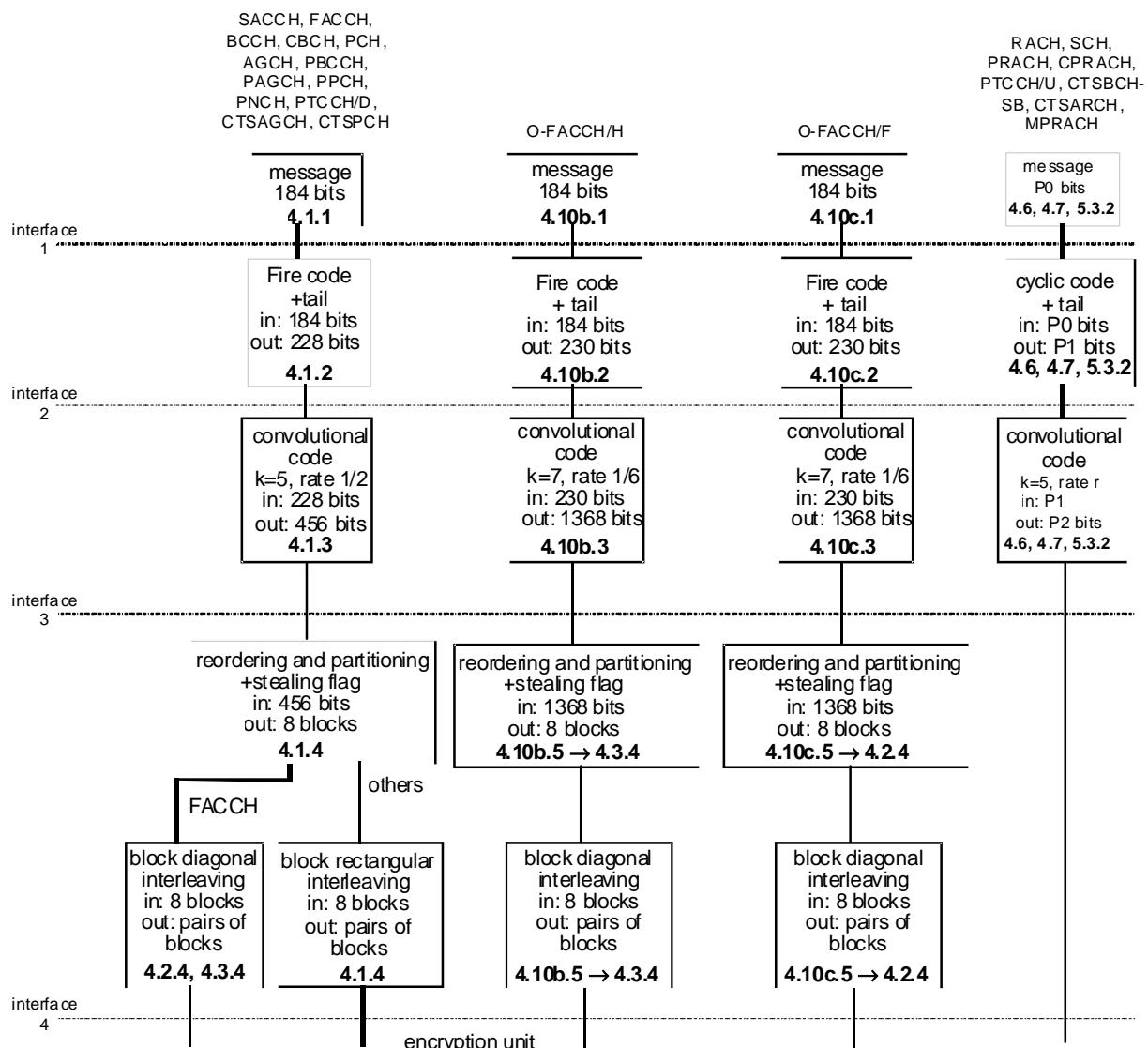
**Figure 2: Channel Coding and Interleaving Organization for control channels except PACCH, EC-BCCCH, EC-SCH, EC-CCCH and EC-PACCH**
