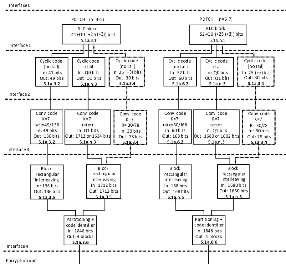
**Figure 1f: Channel Coding and Interleaving Organization for EGPRS2-A Uplink Packet Data Channels**
