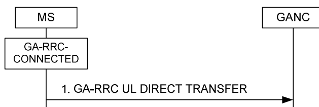
Figure 8a.2.3.1 Uplink direct transfer, normal flow
