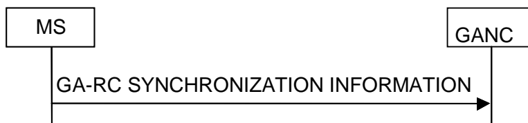
Figure 6.6.1 MS initiated synchronization procedure
