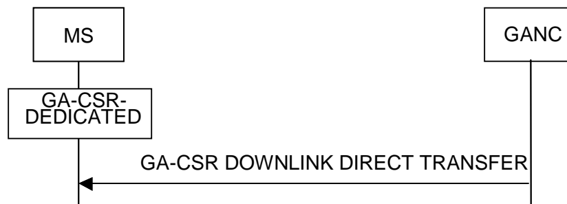
Figure 7.2.3.1 Downlink Direct Transfer, normal flow
