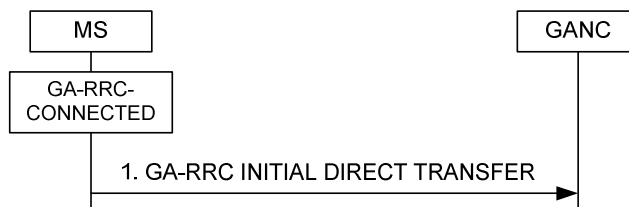
Figure 8a.2.1.1 Initial direct transfer, normal flow
