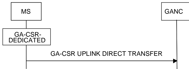
Figure 7.2.1.1 Uplink Direct Transfer, normal flow
