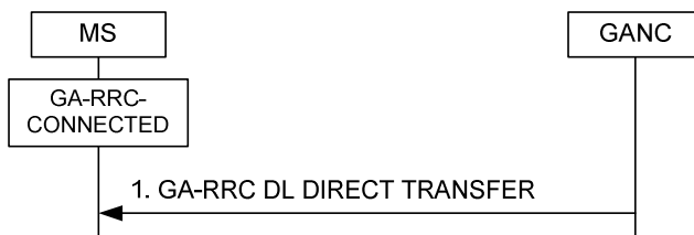
Figure 8a.2.5.1 Downlink direct transfer, normal flow
