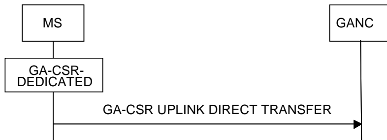
Figure 7.2.1.1 Uplink Direct Transfer, normal flow
