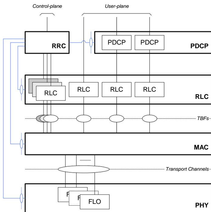
Figure 4.2: Radio Interface Protocol architecture with FLO only
