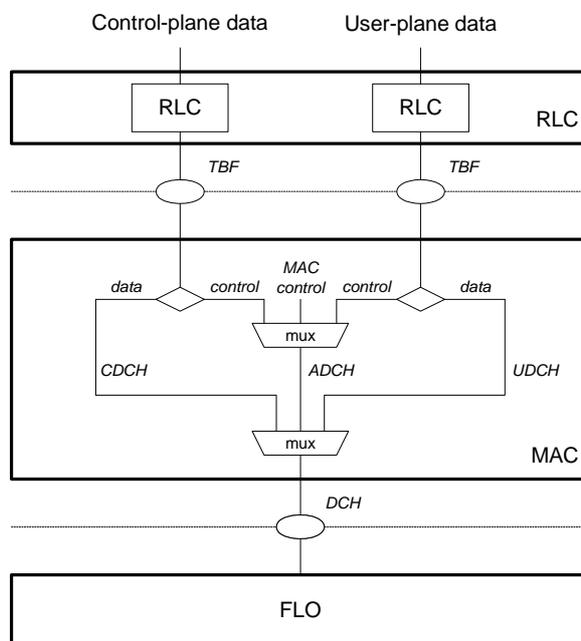
Figure 5.7.2.1: Control-plane and user-plane multiplexing on transport channels
