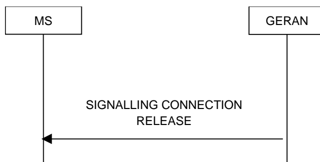
Figure 7.15.1.1.1: Signalling Connection Release procedure, normal case
