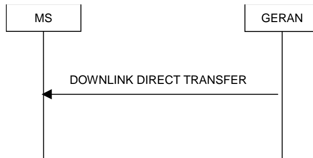
Figure 7.17.2.1: Downlink Direct transfer, normal flow
