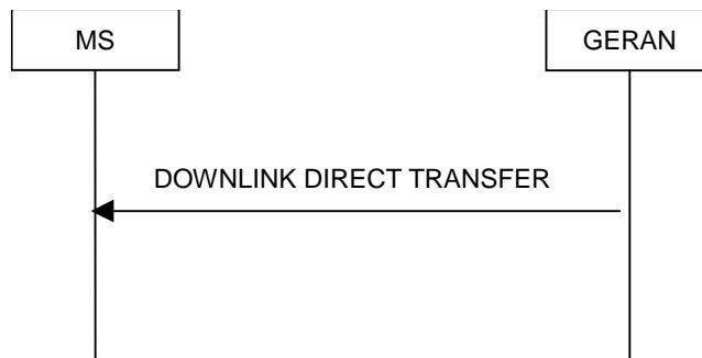
**Figure 7.17.2.1: Downlink Direct transfer, normal flow**
