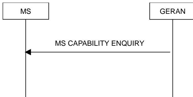
**Figure 7.7.1.1: MS Capability Enquiry procedure, normal flow**
