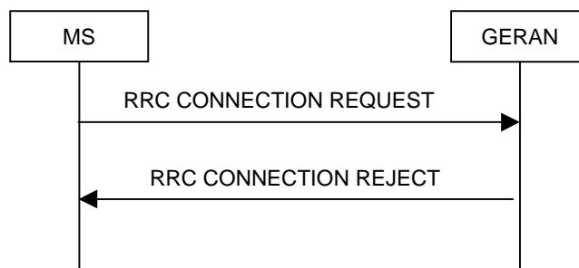
**Figure 7.5.1.2: RRC Connection Establishment, network rejects RRC connection**
