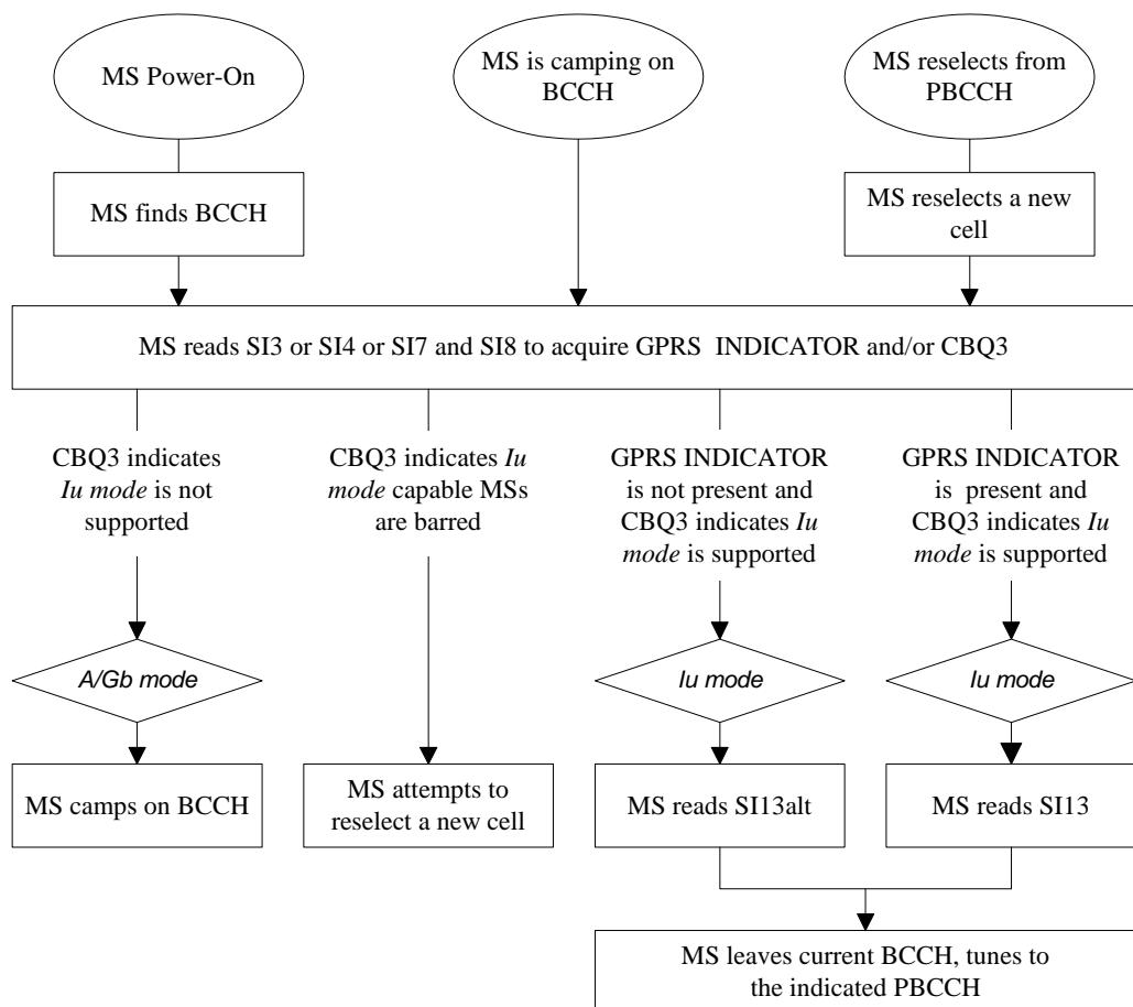
**Figure 7.3.2.2: Behaviour of A/Gb and Iu modes capable MS on BCCH.**
