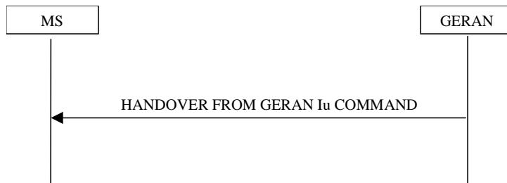
**Figure 7.8.4.1.1: Inter-mode handover from GERAN, successful case**
