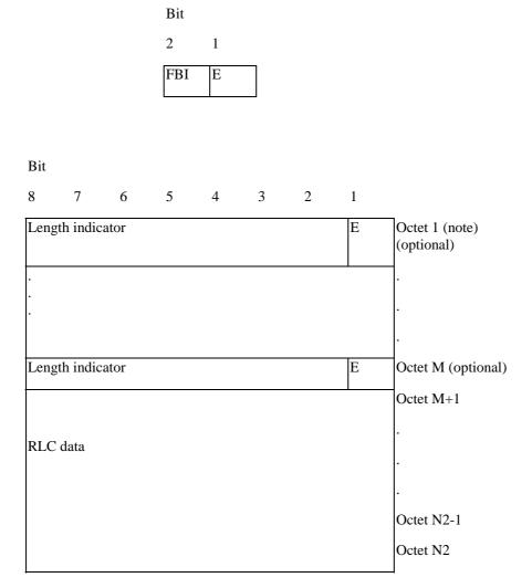
NOTE: If padding is used, then "Octet 1" shall be replaced by "Octet 7", see example in annex J.
