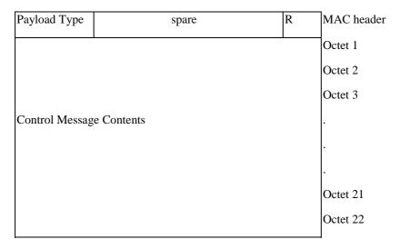
Figure 10.3.2.1: Uplink RLC/MAC control block together with its MAC header
