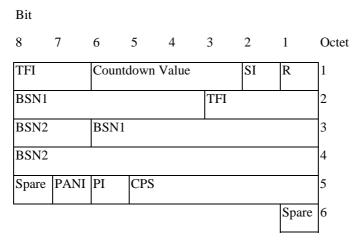
Figure 10.3a.4.4.1: Combined uplink RLC data block header for UAS-7, UAS-8 and UAS-9.
