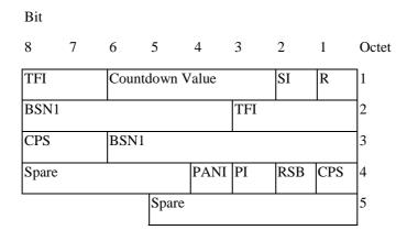
Figure 10.3a.4.2.2: EGPRS uplink RLC data block header (FANR activated) for MCS-5 and MCS-6
