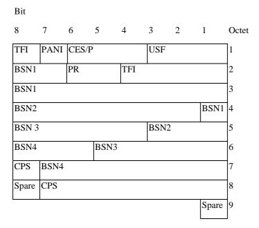
Figure 10.3a.3.9.1: Combined downlink RLC data block header for DBS-11 and DBS-12.
