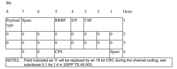
Figure 10.3a.3.3: Downlink RLC/MAC control block header for MCS-0.
