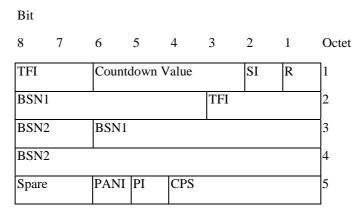
Figure 10.3a.4.7.1: Combined uplink RLC data block header for UBS-7, UBS-8.
