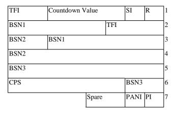
Figure 10.3a.4.8.1: Combined uplink RLC data block header for UBS-9, UBS-10.
