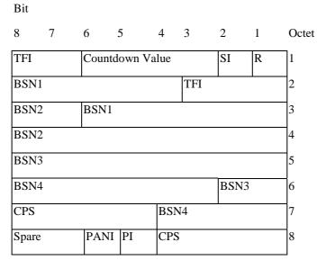
Figure 10.3a.4.9.1: Combined uplink RLC data block header for UBS-11, UBS-12.
