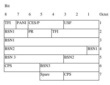
Figure 10.3a.3.8.1: Combined downlink RLC data block header for DBS-9 and DBS-10.
