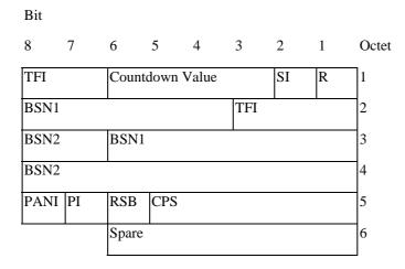
Figure 10.3a.4.1.2: EGPRS uplink RLC data block header (FANR activated) for MCS-7, MCS-8 and MCS-9.
