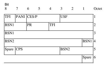
Figure 10.3a.3.7.1: Combined downlink RLC data block header for DBS-7 and DBS-8.
