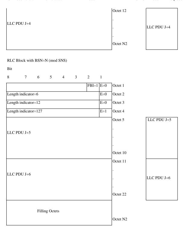
Figure B.9: Example for the case when the LLC PDU fills exactly the RLC data block (LLC PDU J+2 and LLC PDU J+4) and when the last LLC PDU cannot not fill the last RLC data block(LLC PDU J+6)
