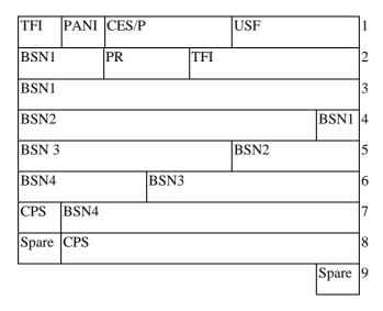
Figure 10.3a.3.9.1: Combined downlink RLC data block header for DBS-11 and DBS-12.
