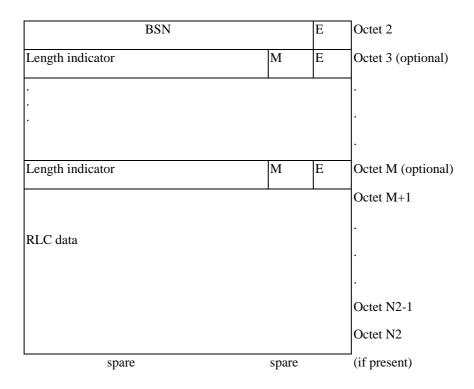
Figure 10.2.1.1: Downlink RLC data block with MAC header
