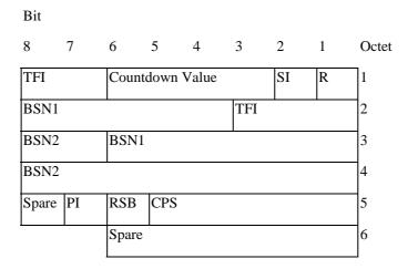
Figure 10.3a.4.1.1: EGPRS uplink RLC data block header (FANR not activated) for MCS-7, MCS-8 and MCS-9.
