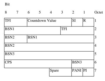
Figure 10.3a.4.5.1: Combined uplink RLC data block header for UAS-10, UAS-11.
