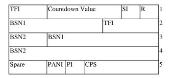
Figure 10.3a.4.7.1: Combined uplink RLC data block header for UBS-7, UBS-8.
