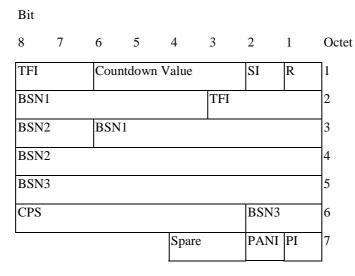
Figure 10.3a.4.8.1: Combined uplink RLC data block header for UBS-9, UBS-10.
