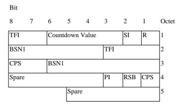
Figure 10.3a.4.2.1: EGPRS uplink RLC data block header (FANR not activated) for MCS-5 and MCS-6
