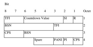
Figure 10.3a.4.6.1: Combined uplink RLC data block header for UBS-5, UBS-6.
