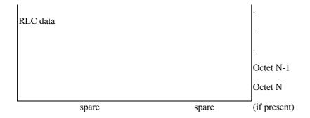
NOTE: The field mapping convention for GPRS (sub-clause 10.0b.3.1) applies. According to that, in particular regarding the TLLI field, the *most significant byte* of the TLLI value shall be mapped on octet M+1 and the *least significant byte* of the TLLI value shall be mapped on octet M+4 of the uplink RLC data block.
