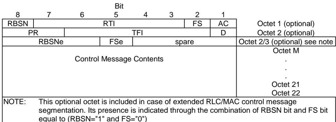
Figure 10.3.1.2: Downlink RLC/MAC control block message contents
