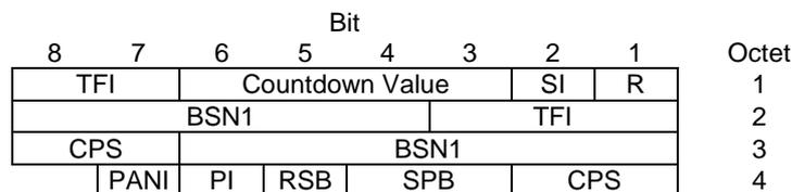
**Figure 10.3a.4.3.2: EGPRS (with FANR)/EGPRS2 uplink RLC data block header for MCS-1, MCS-2, MCS-3 and MCS-4.**
