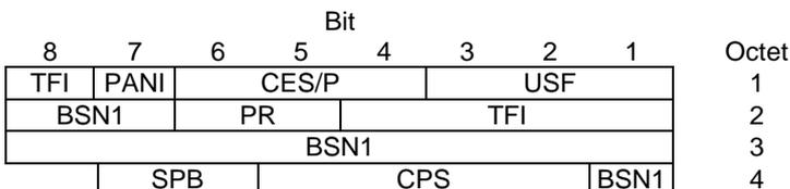
**Figure 10.3a.3.3.2: EGPRS (with FANR)/EGPRS2 downlink RLC data block header for MCS-1, MCS-2, MCS-3 and MCS-4.**
