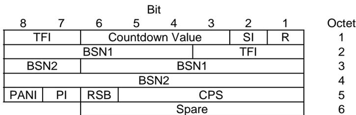
**Figure 10.3a.4.1.2: EGPRS uplink RLC data block header using FANR for MCS-7, MCS-8 and MCS-9.**
