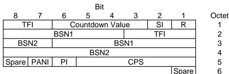
**Figure 10.3a.4.4.1: Combined uplink RLC data block header for UAS-7, UAS-8 and UAS-9.**
