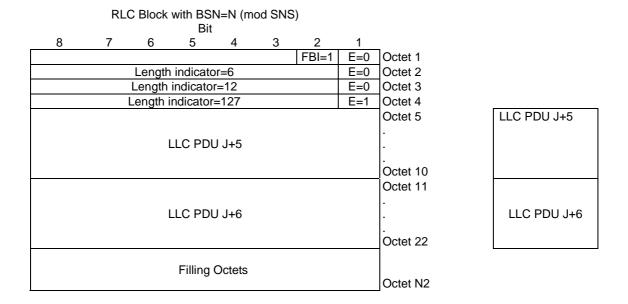
Figure B.9: Example for the case when the LLC PDU fills exactly the RLC data block (LLC PDU J+2 and LLC PDU J+4) and when the last LLC PDU cannot not fill the last RLC data block(LLC PDU J+6)
