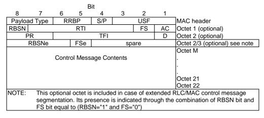
Figure 10.3.1.1: Downlink RLC/MAC control block together with its MAC header
