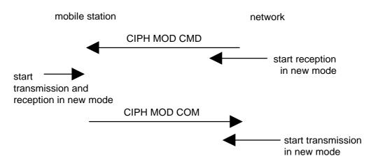
Figure 3.4.7.2.1: Ciphering mode setting sequence
