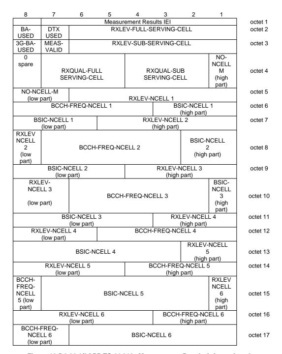
Figure 10.5.2.20.1/3GPP TS 44.018: Measurement Results information element
