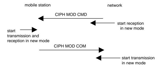
Figure 3.4.7.2.1/3GPP TS 44.018: Ciphering mode setting sequence
