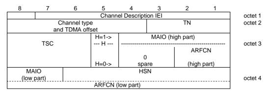
Figure 10.5.2.5a.1/3GPP TS 44.018: Channel Description 2 information element
