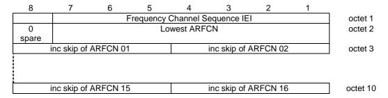
Figure 10.5.2.12.1/3GPP TS 44.018: Frequency Channel Sequence information element
