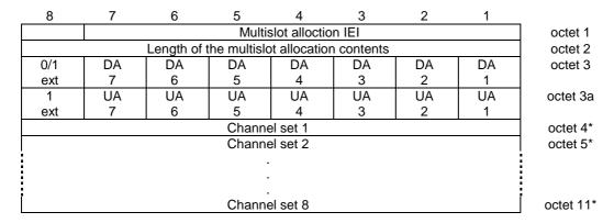
Figure 10.5.2.21b.1/3GPP TS 44.018: Multislot Allocation information element
