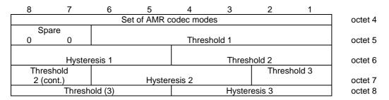
Figure 10.5.2.21aa.5/3GPP TS 44.018: Parameters for multirate speech field for the Multirate speech versions 1 & 2 when a set of four modes is chosen
