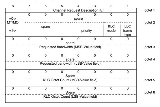
Figure 10.5.2.8a.1/3GPP TS 44.018: Channel Request Description information element
