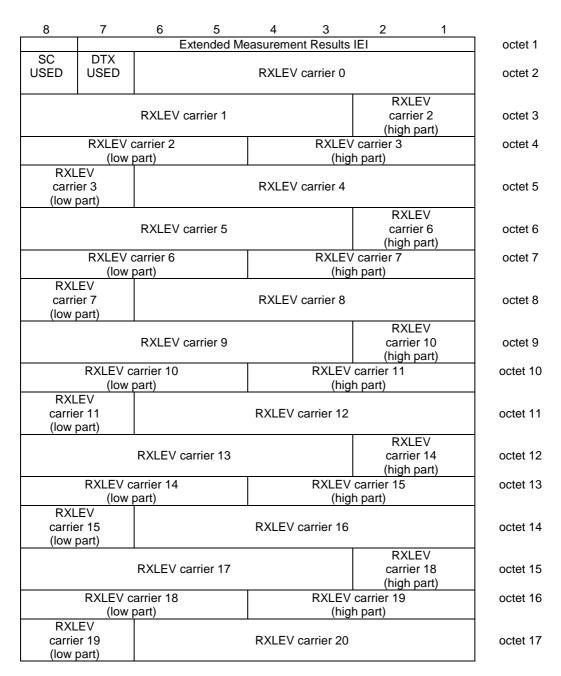
Figure 10.5.2.45.1/3GPP TS 44.018: Extended Measurement Results information element
