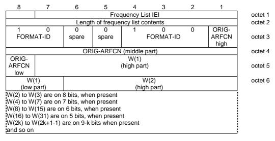
Figure 10.5.2.13.4.1/3GPP TS 44.018: Frequency List information element (Range 512 format)
