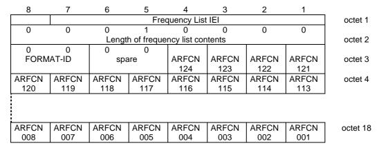
Figure 10.5.2.13.2.1/3GPP TS 44.018: Frequency List information element, bit map 0 format
