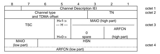
Figure 10.5.2.5.1/3GPP TS 44.018: Channel Description information element
