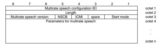
Figure 10.5.2.21aa.1/3GPP TS 44.018: MultiRate configuration information element
