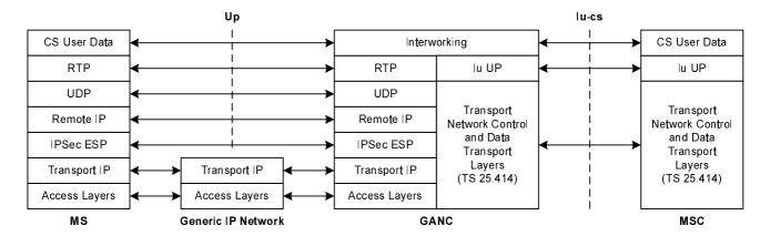
Figure 7c: CS Domain User Plane Protocol Architecture
