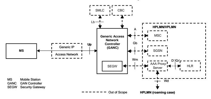
Figure 1: GAN A/Gb mode functional architecture
