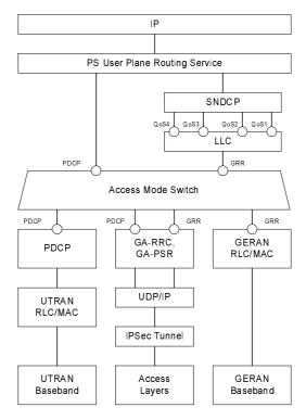
Figure 7h: MS PS Domain User Plane Architecture
