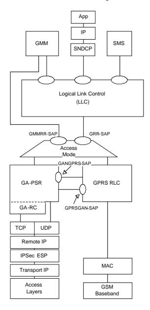
Figure 7: MS PS Domain Architecture
