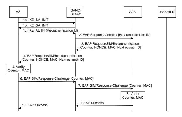
Figure A.3: EAP-SIM fast re-authentication procedure
