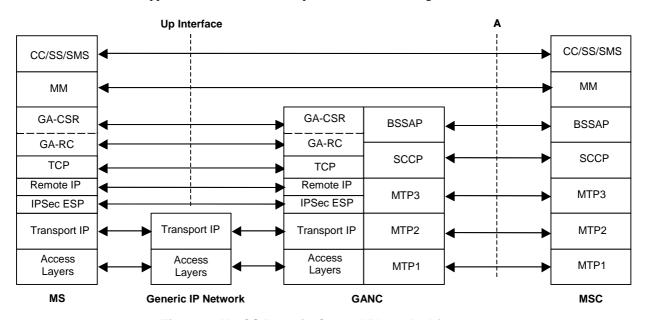
Figure 2: Up CS Domain Control Plane Architecture
