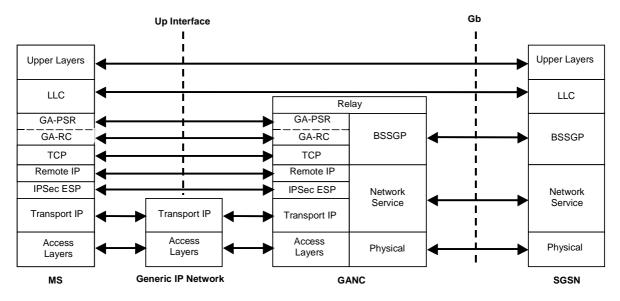
Figure 5: Up PS Domain Control Plane Architecture
