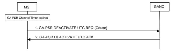
Figure 30: Deactivation of GA-PSR Transport Channel
