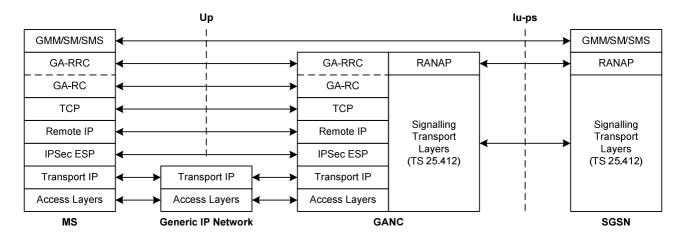
Figure 7e: PS Domain Control Plane Architecture
