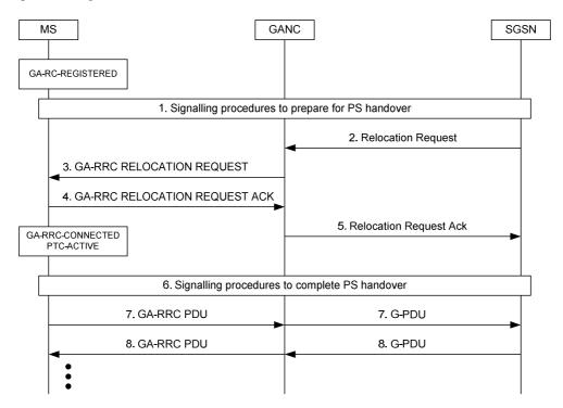
Figure 59a: PTC activation based on Relocation Request
