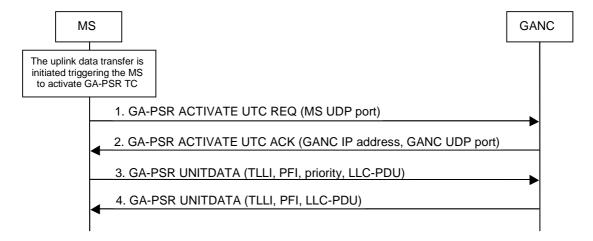
Figure 29: Activation of GA-PSR Transport Channel
