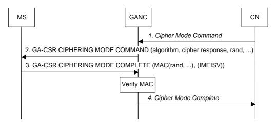
Figure 19: Ciphering Configuration
