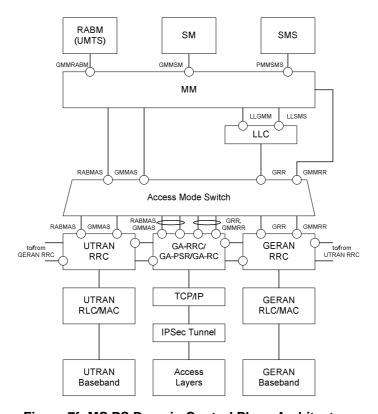
Figure 7f: MS PS Domain Control Plane Architecture
