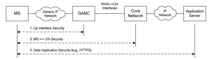
Figure 9: GAN Security Mechanisms
