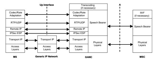
Figure 4: Up CS Domain User Plane Protocol Architecture
