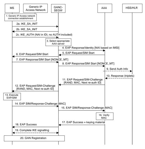
Figure A.1: EAP-SIM authentication procedure
