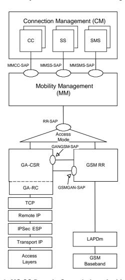
Figure 3: MS CS Domain Control plane Architecture
