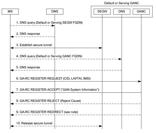
NOTE: The GA-RC REGISTER REDIRECT message may contain: a single Serving SEGW and GANC address or a list of PLMN identities and associated Serving SEGW and GANC addresses; and an Indication of whether GANC address(es) can be stored in the MS for future use.
