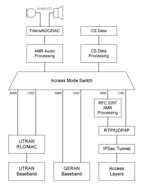
Figure 7d: MS CS Domain User Plane Architecture
