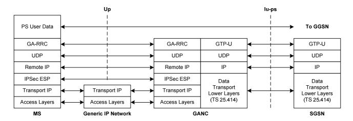
Figure 7g: PS Domain User Plane Protocol Architecture
