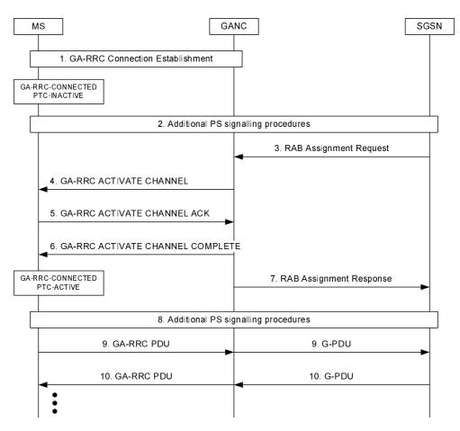
Figure 59: PTC activation based on RAB Assignment Request
