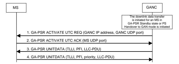
Figure 31: Network initiated GA-PSR Transport Channel Activation
