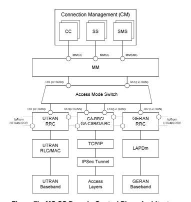
Figure 7b: MS CS Domain Control Plane Architecture
