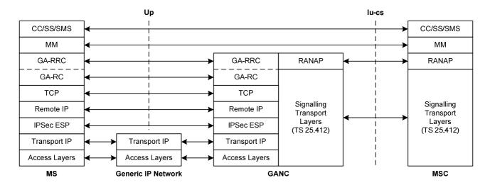
Figure 7a: CS Domain Control Plane Architecture
