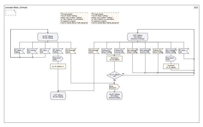
Figure 1a: Handling of Mute/Unmute Requests in Anchor MSC (Sheet 3 of 3)
