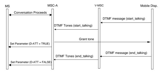
Figure 5d: Signalling information required when the talker is attached to the Anchor MSC and a mobile dispatcher who is roaming in a non-Anchor MSC area sends DTMF signals
