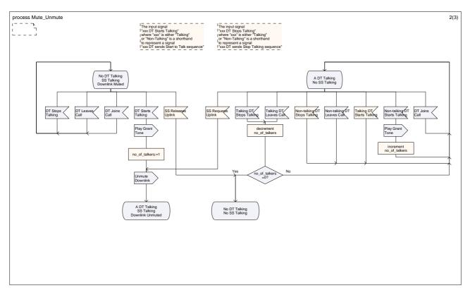
Figure 1a: Handling of Mute/Unmute Requests in Anchor MSC (Sheet 2 of 3)
