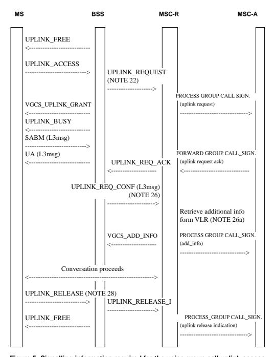
Figure 5: Signalling information required for the voice group call uplink access in the relay MSC without talker priority (normal case, without contention resolution)
