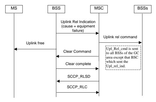
NOTE: The messages CLEAR CMD, CLEAR COM, etc., are used to release the radio and terrestrial resources for the cell serving the talker. The same message flow applies for all cause values different from "call control", and "radio interface failure".
