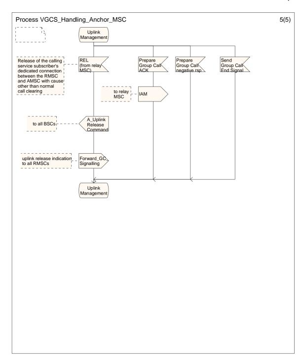
Figure 8: The VGCS handling process in the anchor MSC (sheet 5 of 5)
