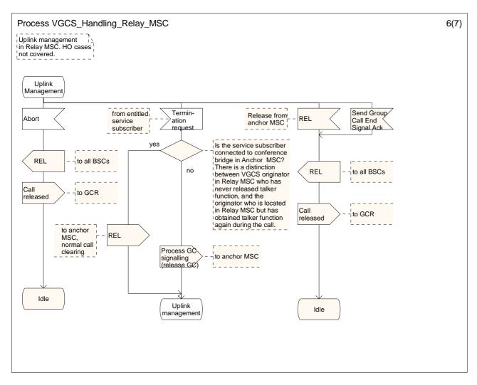
Figure 10: The VGCS handling process in the relay MSC (sheet 6 of 7)
