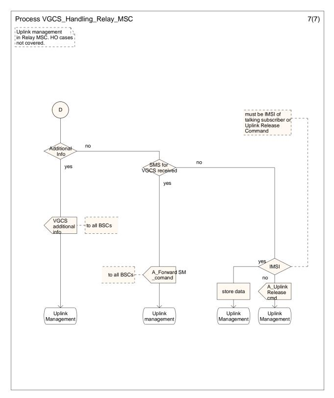
Figure 10: The VGCS handling process in the relay MSC (sheet 7 of 7)
