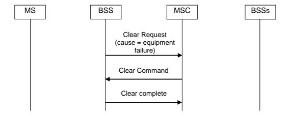
Figure 6.j: A-interface link sharing used or group call re-establishment by the BSS supported:
