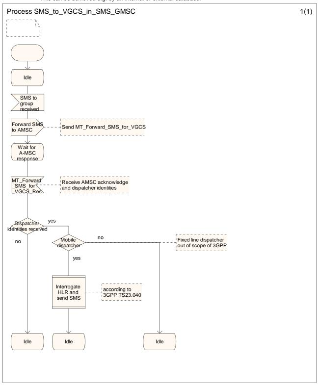
Figure 13: The process in the SMS-GMSC (sheet 1 of 1)
