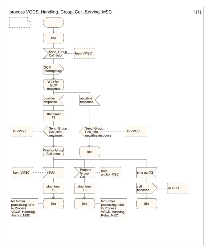
Figure 10A1: The VGCS handling process in the group call serving MSC (sheet 1 of 1)
