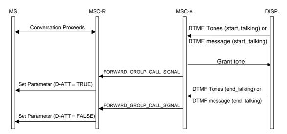
Figure 5c: Signalling information required when the talker is attached to a Relay MSC and a dispatcher sends DTMF signals
