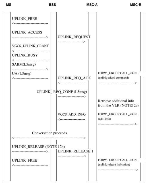
Figure 4: Signalling information required for the voice group call uplink access in the anchor MSC without talker priority (normal case, without contention resolution)
