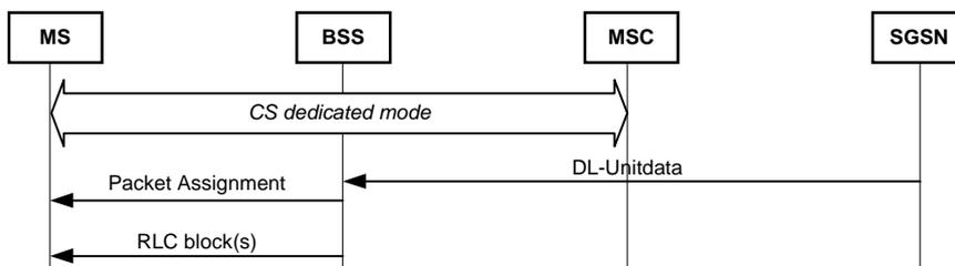
**Figure 7: Example of a successful establishment of a PS MT session while in dedicated mode, packet idle mode and Ready state**
