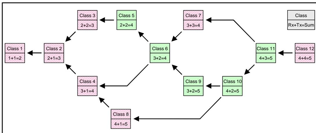
Figure 19 – Incremental support of multislot classes.
