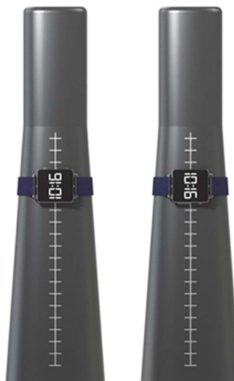
Figure B.3.2.3-2: Left and Right positioning for Wrist-Worn Device on Forearm Phantom (© 2001 – 2022 CTIA Certification. Reproduced with permission.), defined in the CTIA Certification OTA Test Plan
