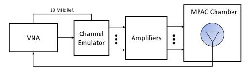
Figure C.3.2-1: Setup for PDP measurements
