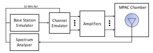
Figure C.3.6-1: Setup for power validation measurements
