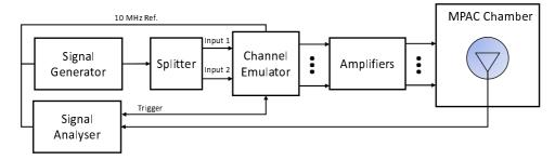
Figure C.3.3-3: Setup for Beam-Specific Doppler measurements (Beam 1)
