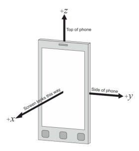
Figure G.3-1: DUT default orientation to coordinate system
