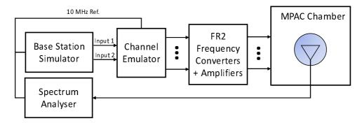
Figure I.3.6-1: Setup for FR2 power validation measurements
