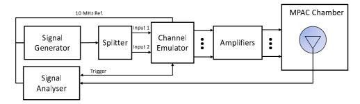
Figure C.3.5-3: Setup for Beam-Specific V/H measurements (Beam 1)
