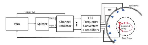
Figure I.3.4-2: Setup for FR2 PSP validation measurements
