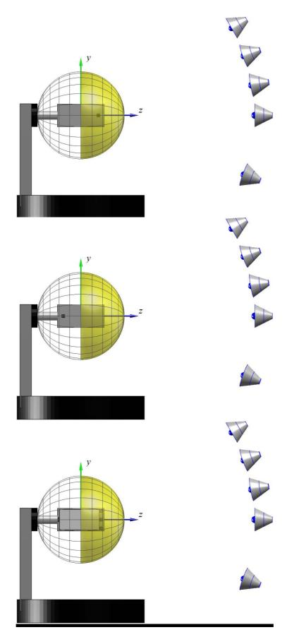
Figure G.3-2: Illustration of DUT re-positioning using a sample FR2 MPAC system. The region with reduced signal ripple is illustrated in yellow
