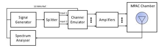
Figure C.3.3-1: Setup for Doppler measurements
