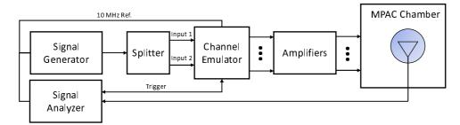
Figure C.3.4-7: Configuration for spatial correlation validation based on time domain techniques (CDL-C UMi)
