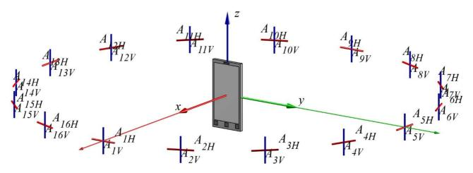
Figure A.2.1-2: OTA chamber antenna setup with sixteen uniformly spaced dual polarized chamber antennas
