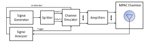
Figure C.3.3-2: Setup for Doppler measurements based on time domain technique
