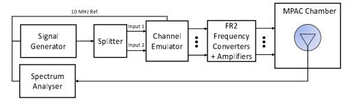
Figure I.3.3-1: Setup for FR2 Doppler measurements
