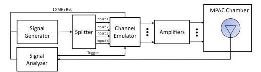
Figure C.3.4-8: Configuration for spatial correlation validation based on time domain techniques (CDL-C UMa)
