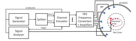
Figure I.3.4-3: Setup for FR2 PSP validation measurements based on time domain
