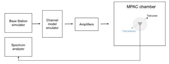
Figure C.3.6-1: Setup for power validation measurements
