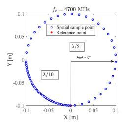
Figure C.3.4-5: Spatial sampling for spatial correlation validation measurement for test frequencies less than and equal to or greater than 1800 MHz: 617 MHz spatial sampling (left) and 4700 MHz spatial sampling (right)
