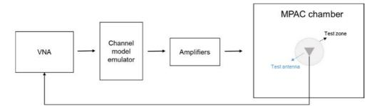
Figure C.3.2-1: Setup for PDP measurements
