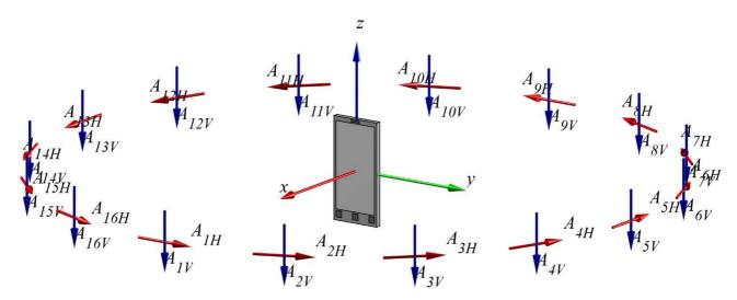
Figure A.2.1-2: OTA chamber antenna setup with sixteen uniformly spaced dual polarized chamber antennas
