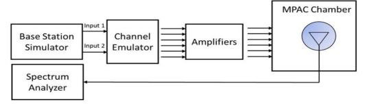
Figure C.3.6-2: Setup for power validation measurements for CDL-C UMi
