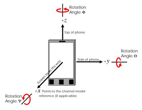
Figure A.4-2: DUT default alignment of example smartphone UE to coordinate system
