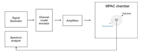
Figure C.3.3-1: Setup for Doppler measurements
