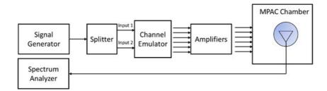
Figure C.3.3-3: Setup for Beam-Specific Doppler measurements (Beam 1)
