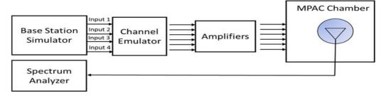
Figure C.3.6-3: Setup for power validation measurements for CDL-C Uma
