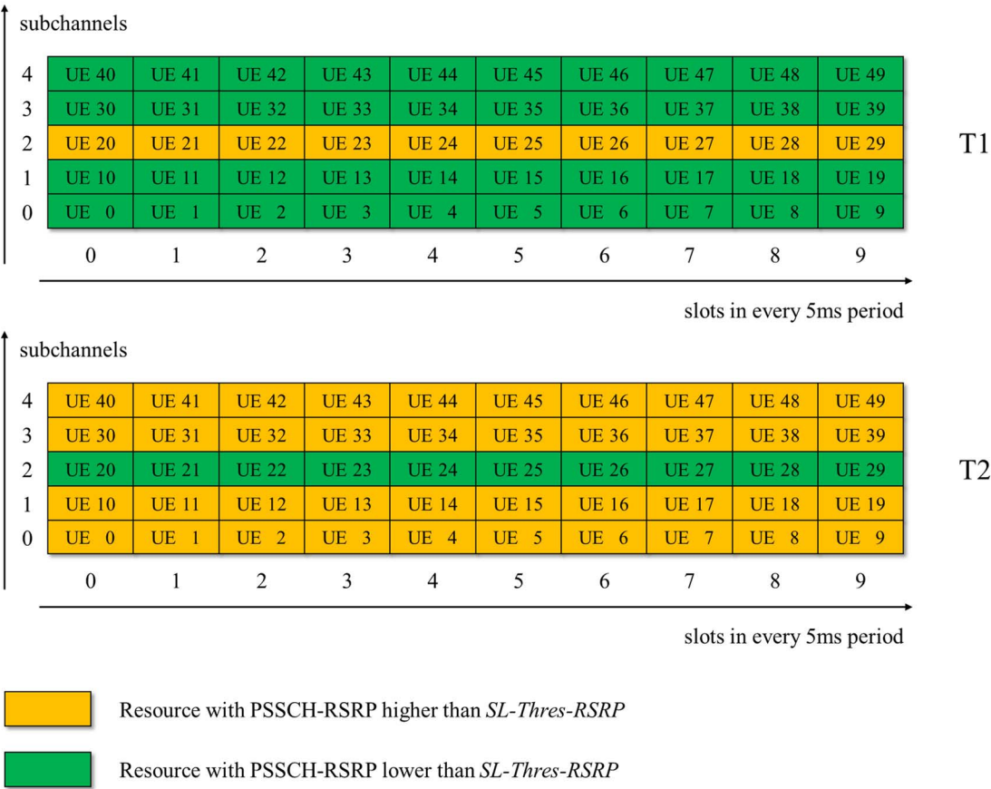
Figure 9.1.4.1.5-2: Power level variation of active sidelink UEs for NR SA FR1 L1 SL-RSRP measurement for autonomous resource selection/reselection
