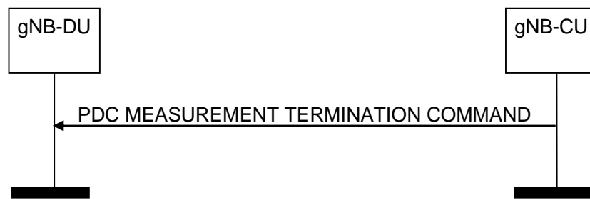
Figure 8.15.3.2-1: PDC Measurement Termination procedure: successful operation
