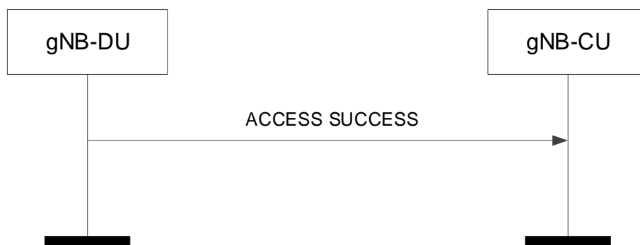
Figure 8.3.8.2-1: Access Success procedure. Successful operation.
