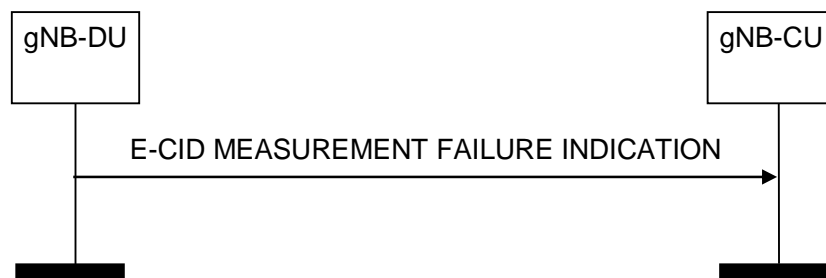
Figure 8.13.13.2-1: E-CID Measurement Failure Indication, successful operation
