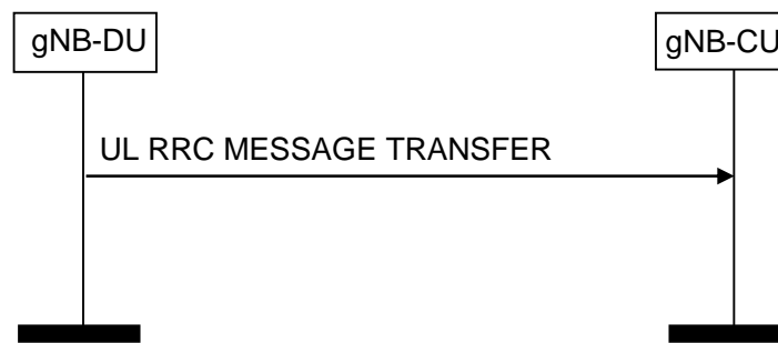
Figure 8.4.3.2-1: UL RRC Message Transfer procedure
