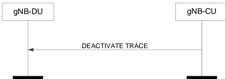
Figure 8.8.2.2-1: Deactivate trace procedure: Successful Operation
