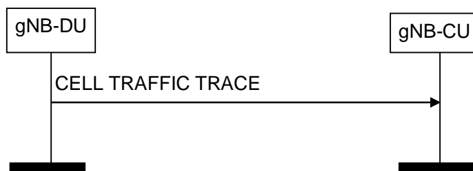
Figure 8.8.3.2-1: Cell Traffic Trace procedure. Successful operation.
