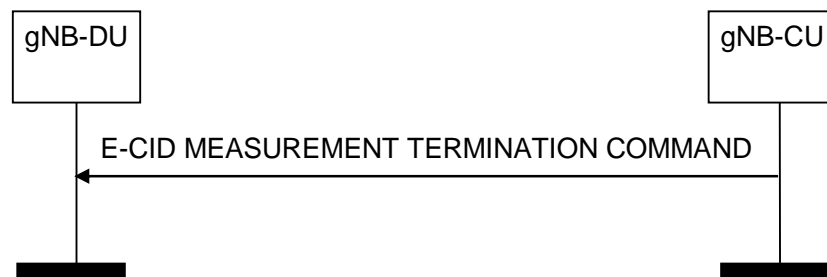
Figure 8.13.15.2-1: E-CID Measurement Termination procedure, successful operation
