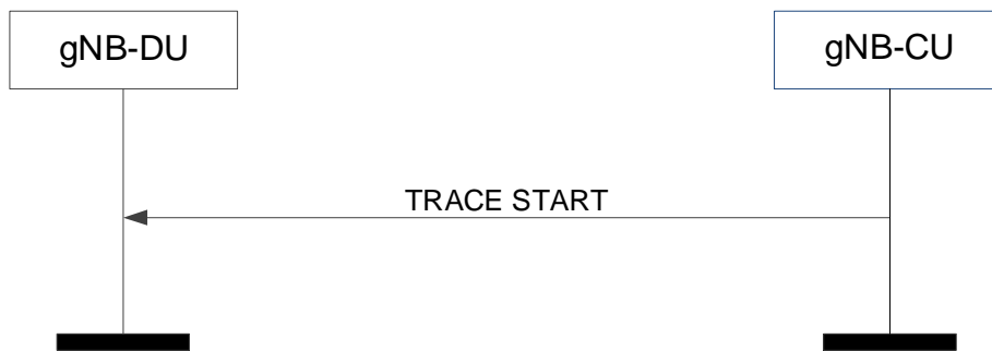
Figure 8.8.1.2-1: Trace start procedure: Successful Operation.
