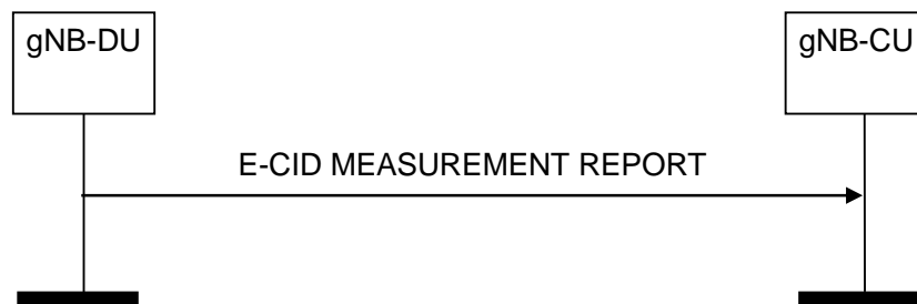
Figure 8.13.14.2-1: E-CID Measurement Report procedure, successful operation
