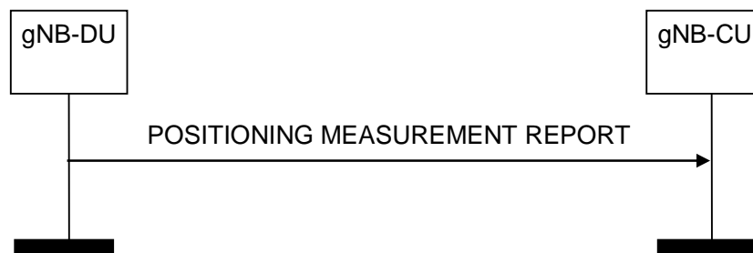
Figure 8.13.4.2-1: Positioning Measurement Report procedure: successful operation
