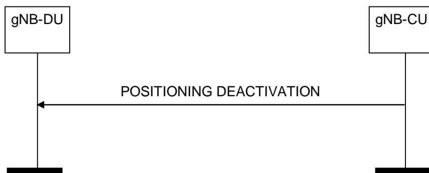
Figure 8.13.11.2-1: Positioning Deactivation procedure, successful operation
