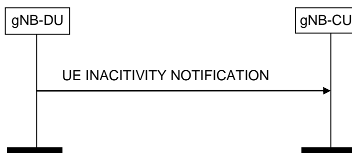
Figure 8.3.6.2-1: UE Inactivity Notification procedure.
