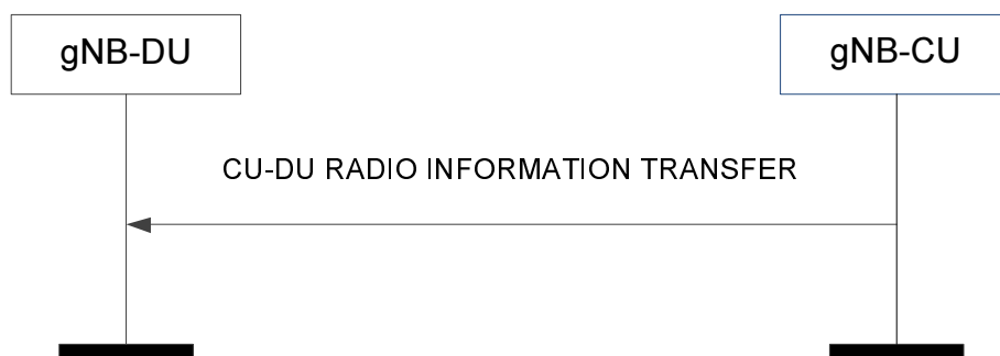
Figure 8.9.2.2-1: CU-DU Radio Information Transfer procedure.
