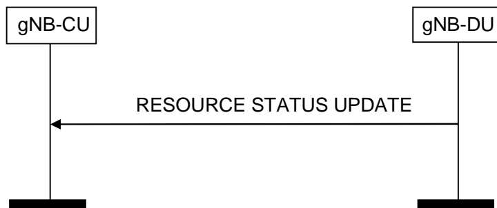
Figure 8.2.11.2-1: Resource Status Reporting, successful operation
