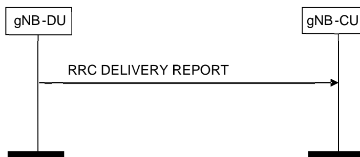
Figure 8.4.4.2-1: RRC Delivery Report procedure.
