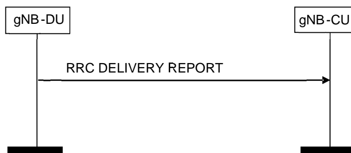
Figure 8.4.4.2-1: RRC Delivery Report procedure.
