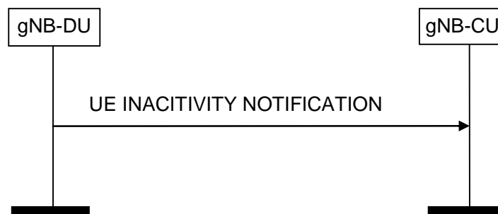
Figure 8.3.6.2-1: UE Inactivity Notification procedure.
