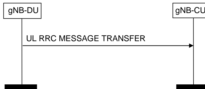
Figure 8.4.3.2-1: UL RRC Message Transfer procedure
