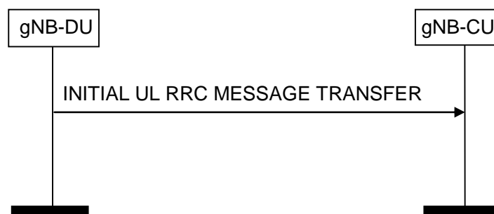
Figure 8.4.1.2-1: Initial UL RRC Message Transfer procedure.
