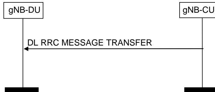
Figure 8.4.2.2-1: DL RRC Message Transfer procedure
