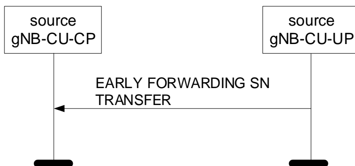
Figure 8.3.12.2-1: Early Forwarding SN Transfer procedure: Successful Operation.
