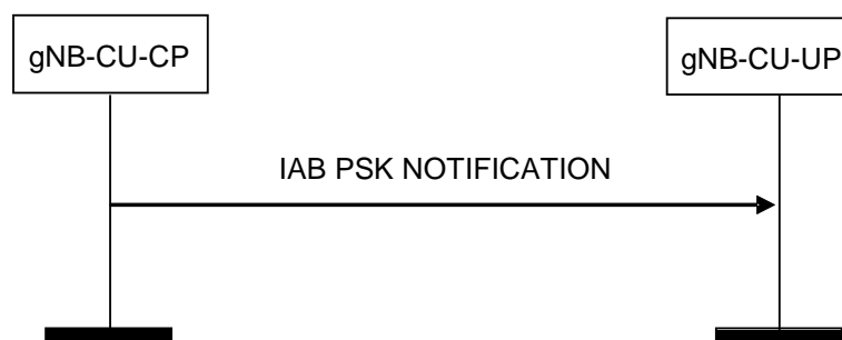
Figure 8.5.2.2-1: IAB PSK Notification procedure: Successful Operation.
