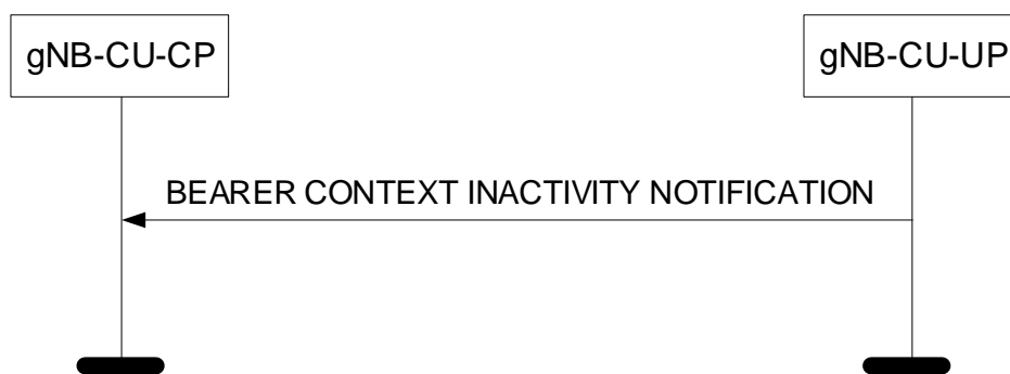
Figure 8.3.6.2-1: Bearer Context Inactivity Notification procedure: Successful Operation.
