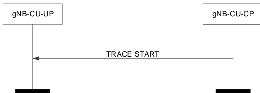
Figure 8.4.1.2-1: Trace start procedure: Successful Operation.
