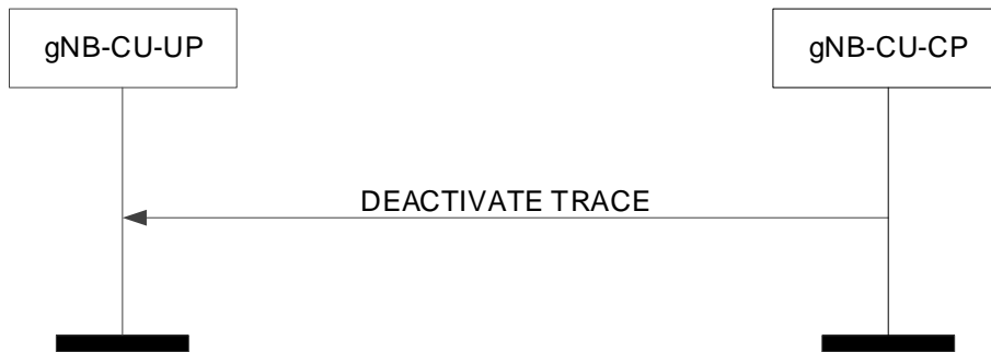
Figure 8.4.2.2-1: Deactivate trace procedure: Successful Operation.
