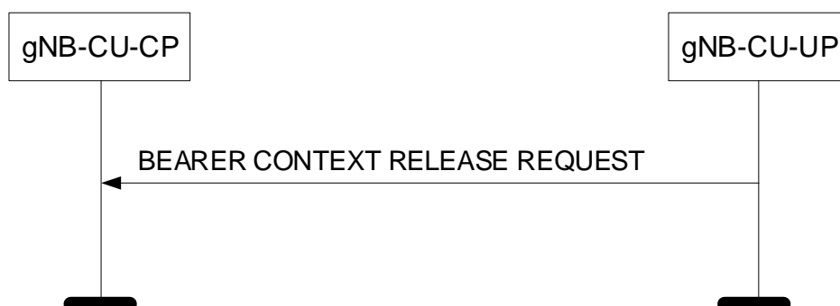
Figure 8.3.5.2-1: Bearer Context Release Request procedure: Successful Operation.
