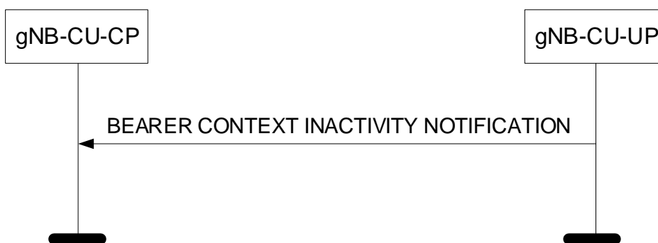
Figure 8.3.6.2-1: Bearer Context Inactivity Notification procedure: Successful Operation.
