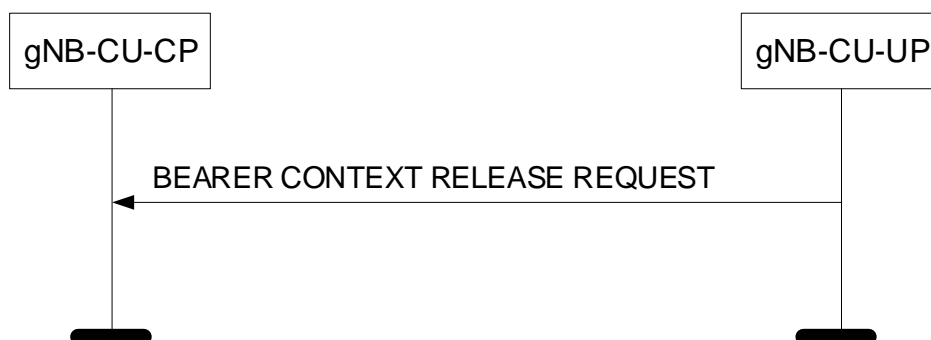
Figure 8.3.5.2-1: Bearer Context Release Request procedure: Successful Operation.
