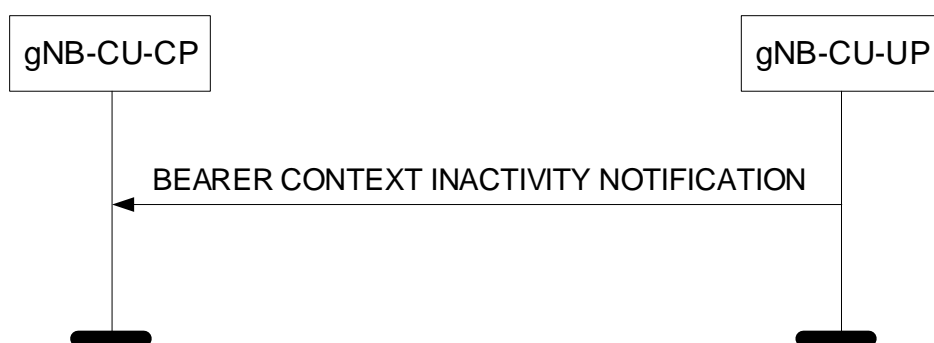
Figure 8.3.6.2-1: Bearer Context Inactivity Notification procedure: Successful Operation.
