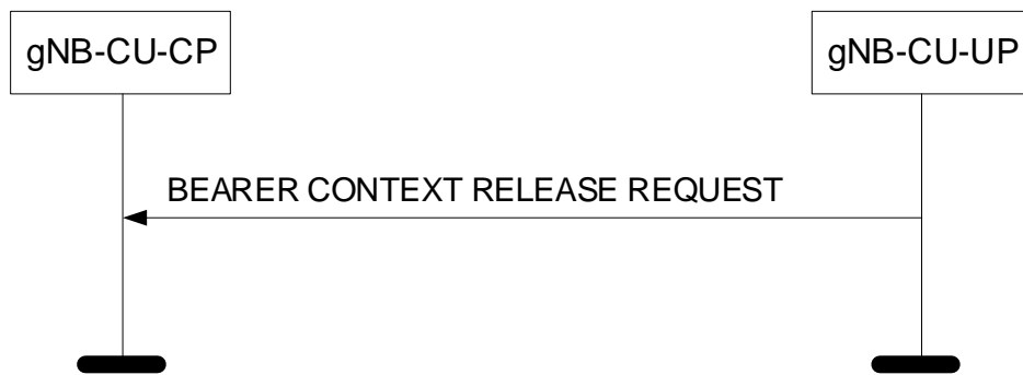
Figure 8.3.5.2-1: Bearer Context Release Request procedure: Successful Operation.
