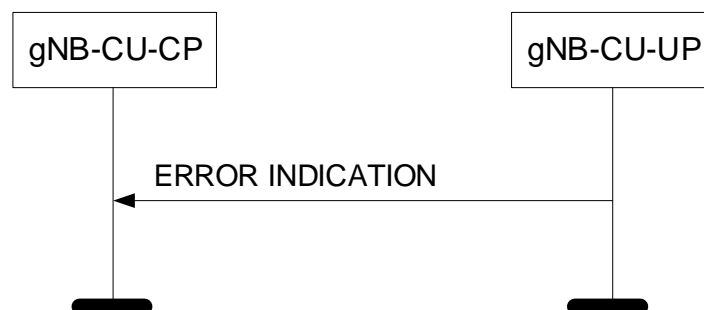
Figure 8.2.2.2-2: Error Indication procedure, gNB-CU-UP originated. Successful operation.
